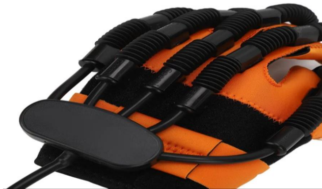
Figure 22: Rehabilitation robot glove for hemiplegic patients
