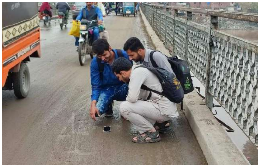
Figure 4-4 Acceleration response measurement using smartphones
