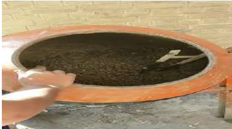
Figure 3.11: Mixing of cement and aggregates with water in a batch mixer
