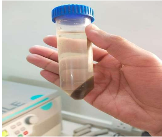
Figure 3.7: Appearance of light brown HGO after washing and centrifugation
