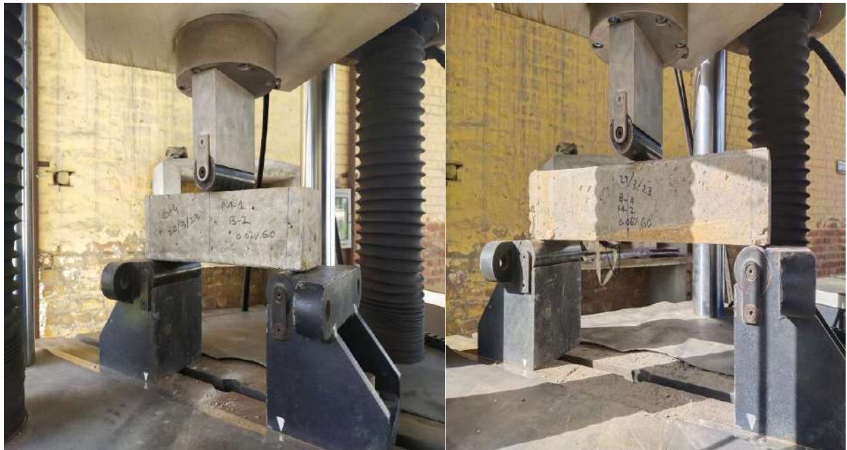
Figure 3.19: Placing specimens into UTM for flexural strength test using simple beam with center-point loading
