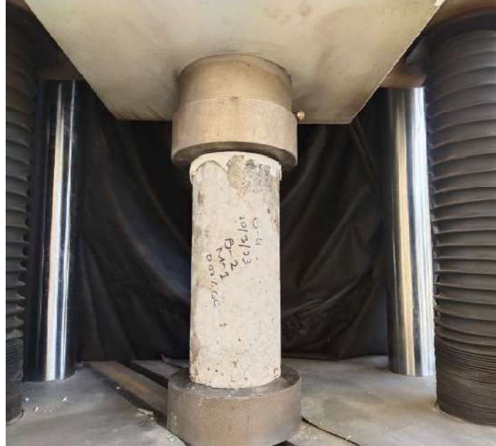
Figure 3.15: Specimen placement to assess specimen compressive behavior
