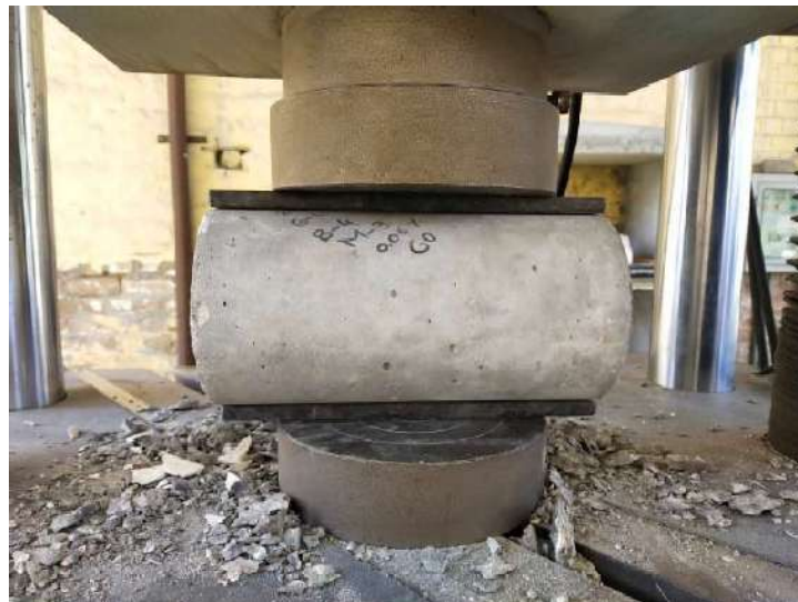
Figure 3.18: Placing specimen into UTM for splitting tensile strength test
