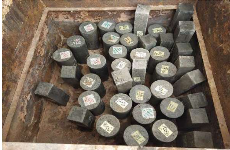
Figure 3.13: Concrete samples in water tank for curing
