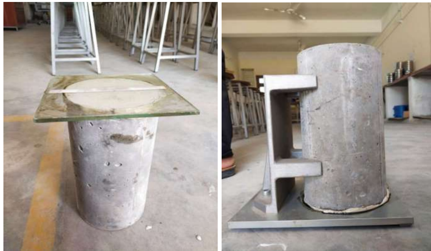
Figure 3.14: Applying Plaster of Paris coating for flat ends
