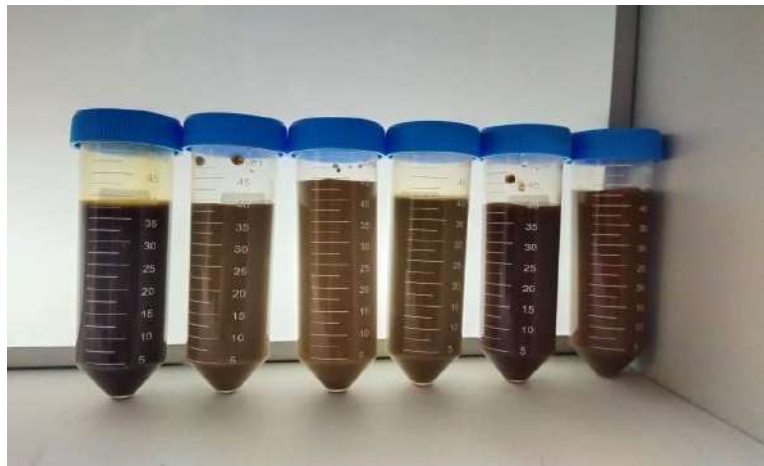
Figure 3.8: Sample of HGO after sonication having concentration of 0.723g for 15 ml
