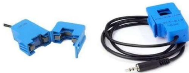
Figure 3: SCT-013 Current Sensor
