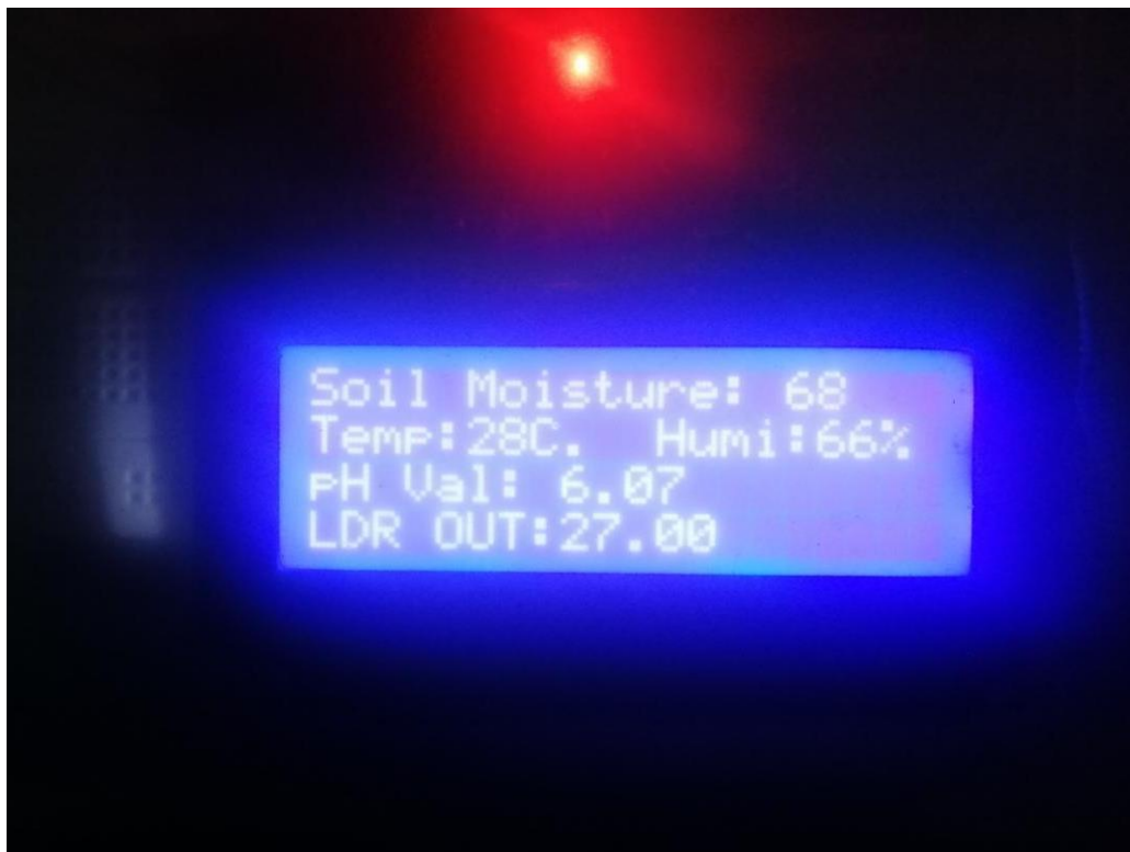
Figure 24: Sensors Values on LCD
