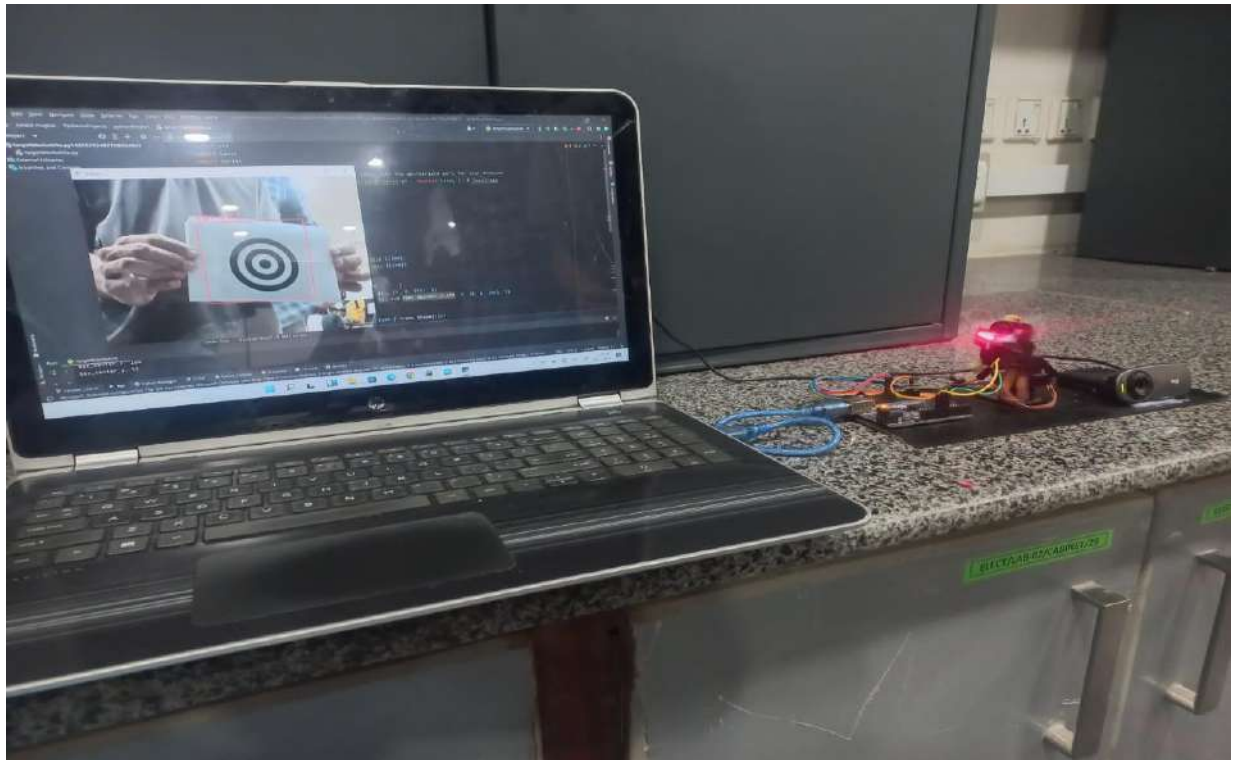
Figure 3.16 Tracking and target locking on Bullseye image as target
