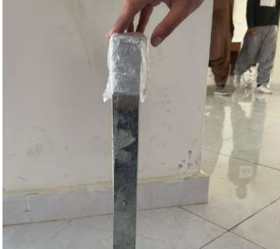
Tubular Column filled with ECC
