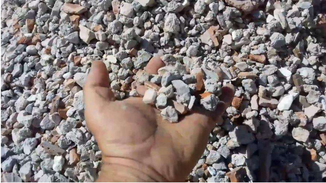
Figure 6: Concrete Used as Aggregates
