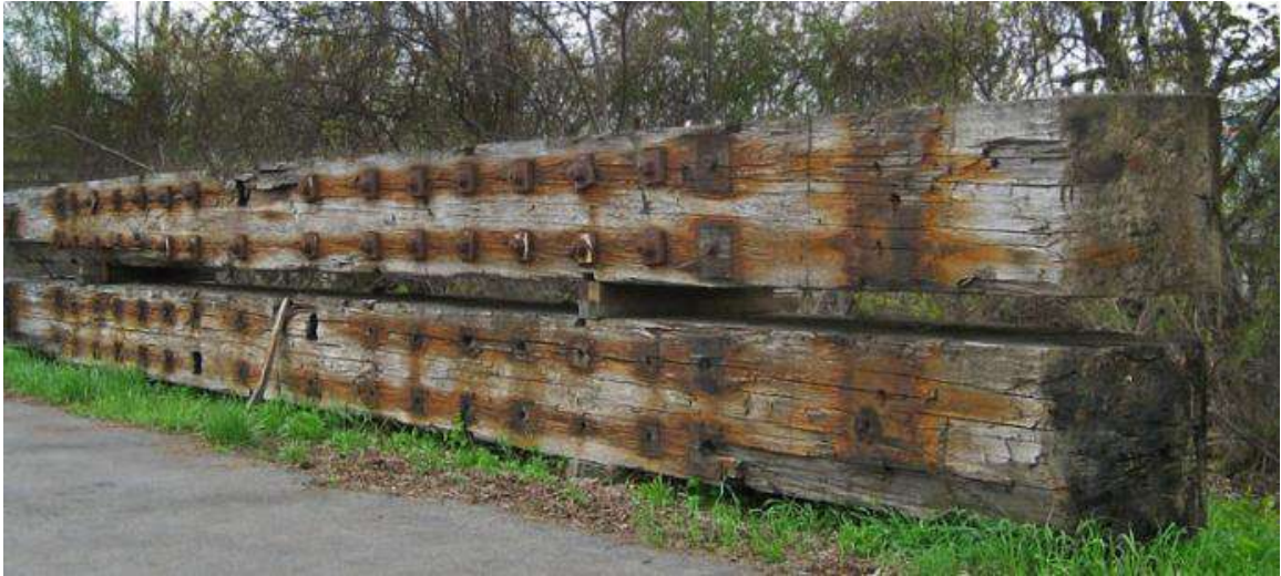
Figure 9: The trees were harvested in the early 1900's, they were 400 years old: 37" * 42" * 48' timbers from Welland Canal Lock.
