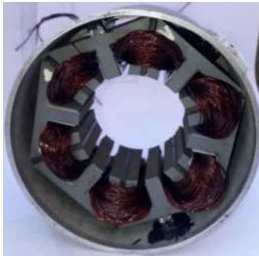
Figure 4.6: Internal view of stator.
