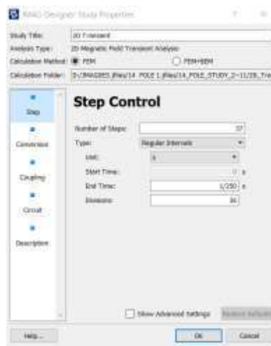
Figure 3.15: Properties for setting End time and steps.
