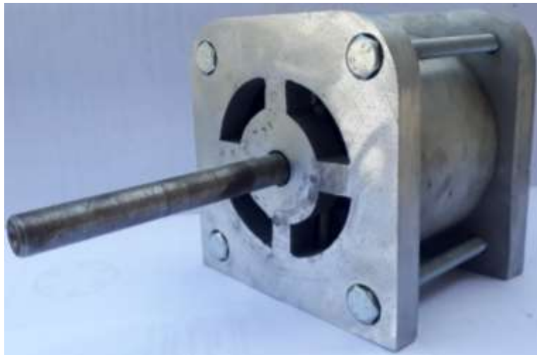
Figure:4.8 Final prototype of hexagonal machine.
