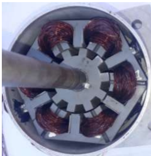
Figure 4.7: Internal view of the hexagonal machine
