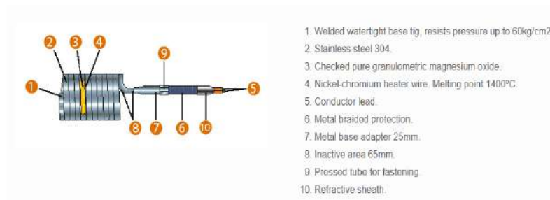
Figure 2.13 Mechanism of coil heater [18]
