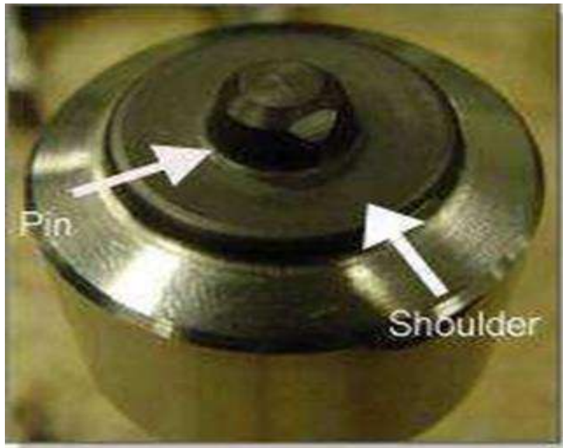
Figure 3.2 Pin and Shoulder of FSW
