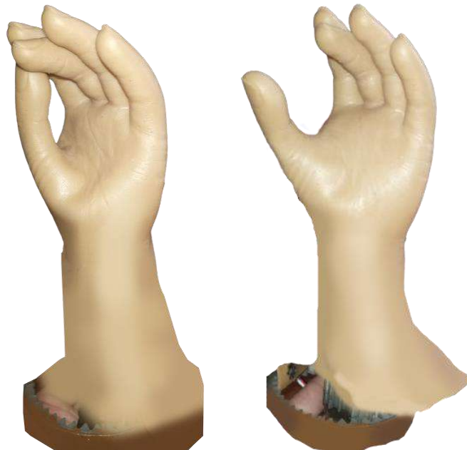
Fig 5.7 Electromechanical prosthetic hand DOF-2 Wrist rotation with gripping
