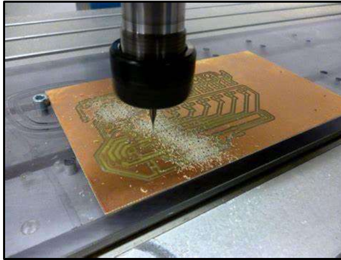
Figure 2-2 PCB Being Fabricated by CNC Milling
