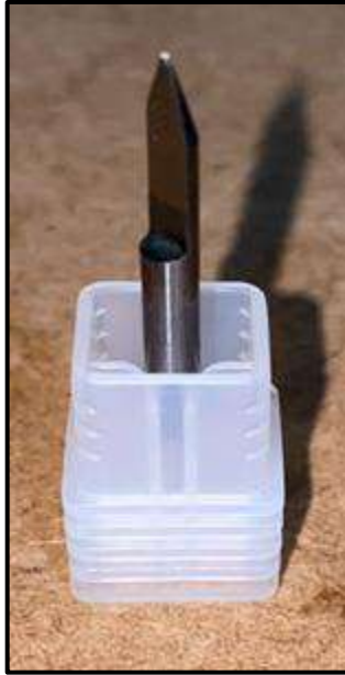
Figure 4-25 Engraving Tool (30 degree, 3.75mm holding diameter, 0.1mm tip diameter)
