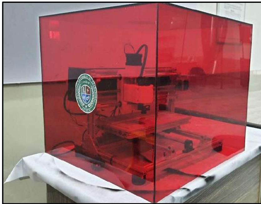
Figure 4-34 Fully fabricated Covered Machine (due to protection from reflected radiation of laser)
