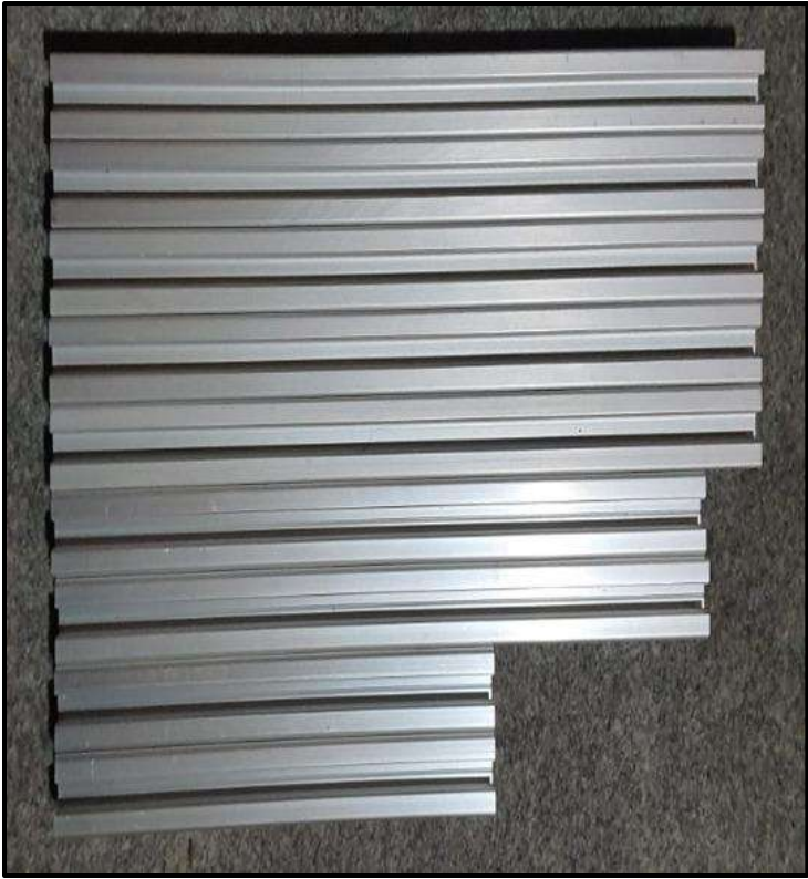
Figure 4-23 Universal 2020 Aluminum Profile for Frame
