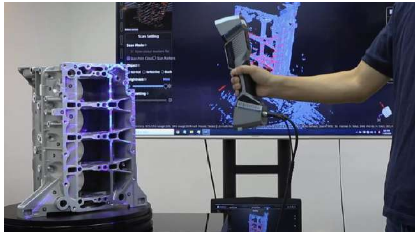
Figure 14 Handheld Blue Laser Scanning Captures 3D Metrology (FreeScan UE 3D Laser Scanner)
