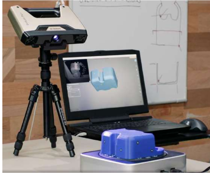
Figure 8 Reverse Engineering Process
