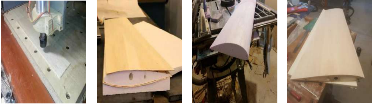
Figure 4.13: CUTTING AND ASSEMBLY OF WINGS
