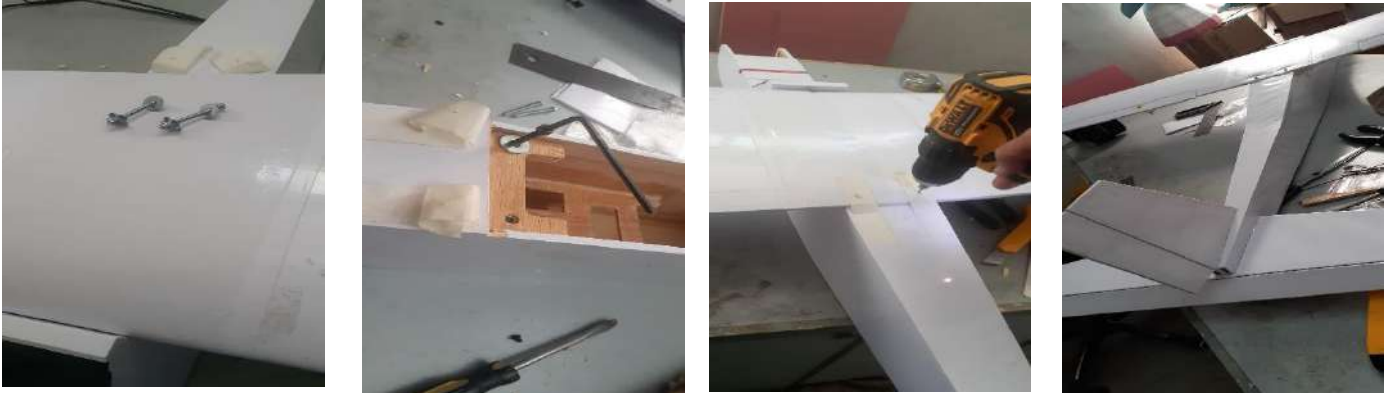
FIGURE 4.17 ATTACHING WINGS TO THE FUSELAGE
