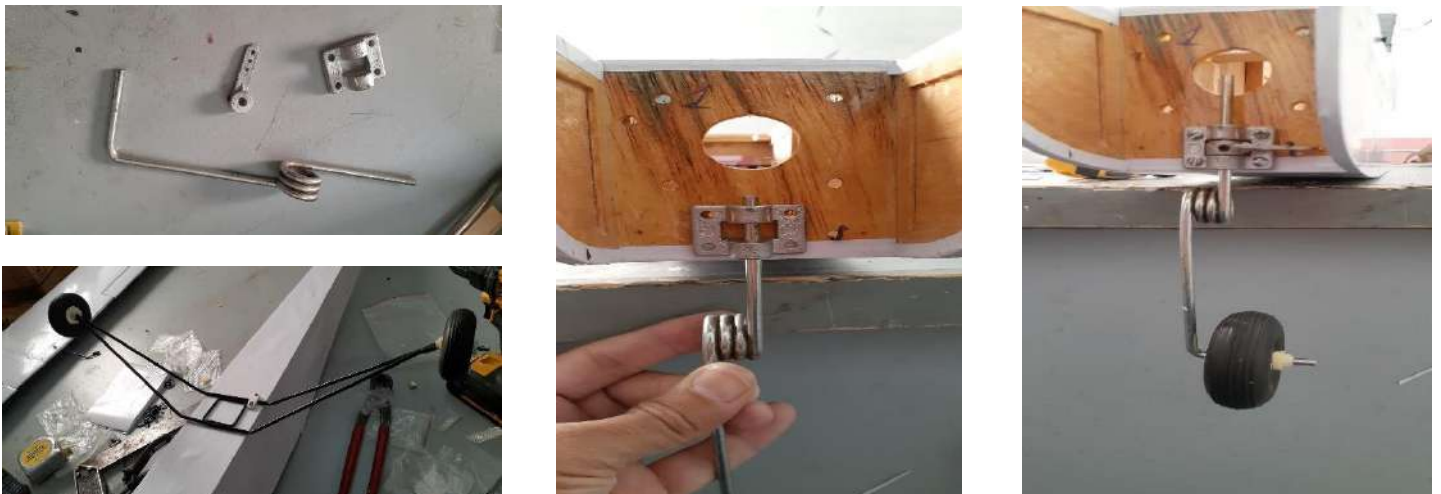
FIGURE 4.19 LANDING GEAR INSTALLING
