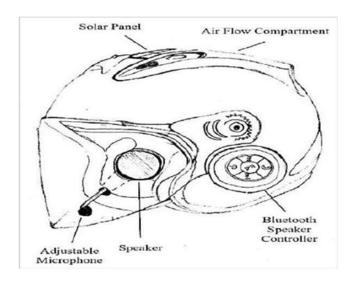
The concept design shown in Figure 1 is a half face helmet with basic equipment such as a helmet visor and an air flow channel. The additional components in the concept design include a pair of mini speakers, a Bluetooth speaker controller with quick access buttons, an adjustable microphone, and a solar panel on the top of the helmet as a power source.
