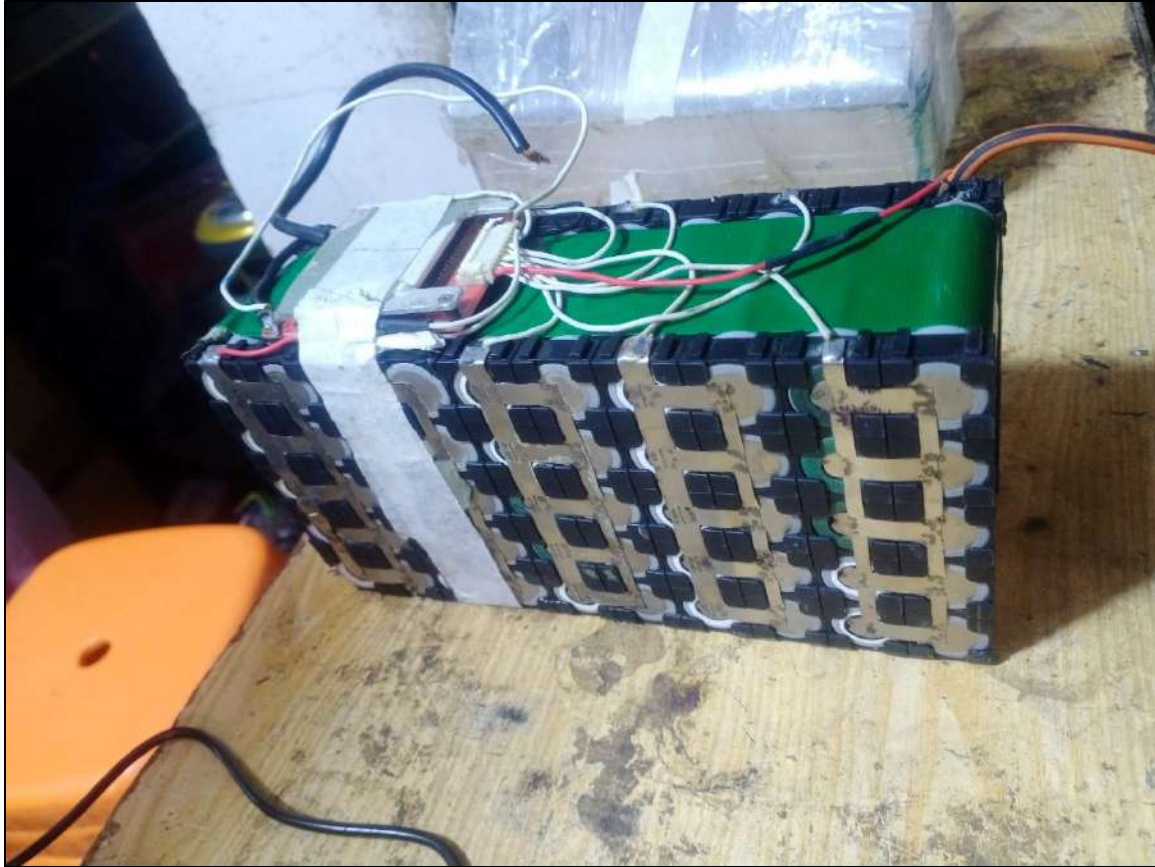
Figure 4. 2: Series and Parallel Connection of Battery
