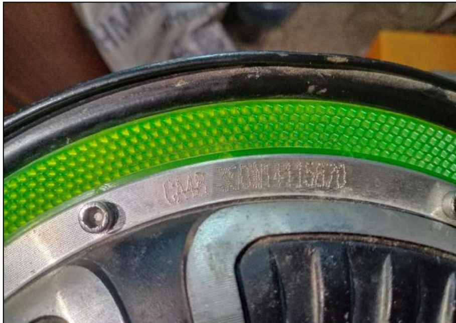
Figure 1. 5: Hub Motor CA48 350W14115870
