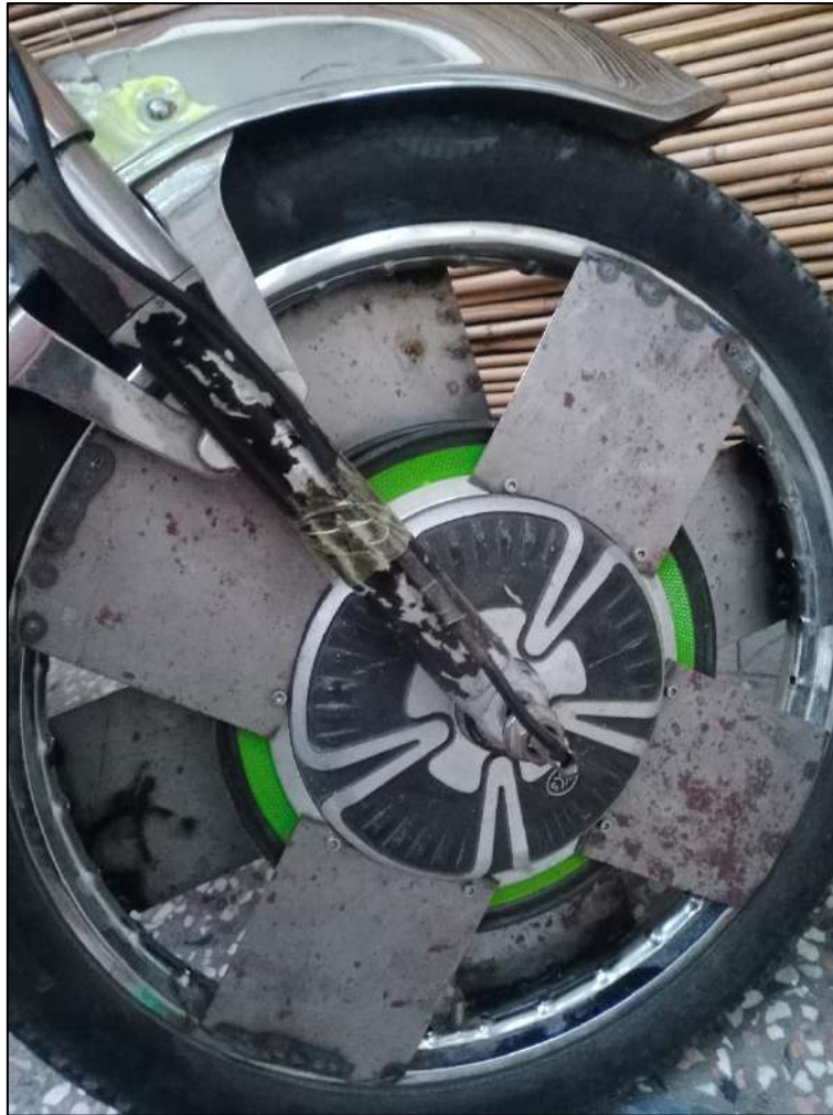
Figure 5. 4: Hub Motor in Front Wheel
