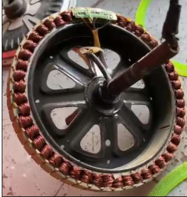
Figure 3. 3 Internal Configuration of Hub Motor
