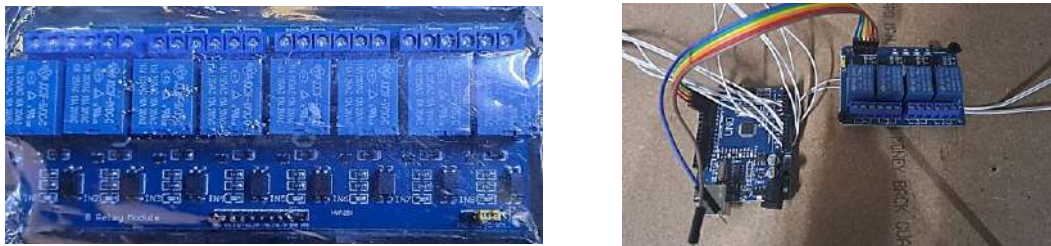
Figure 5-3: Relay Motor Drives
