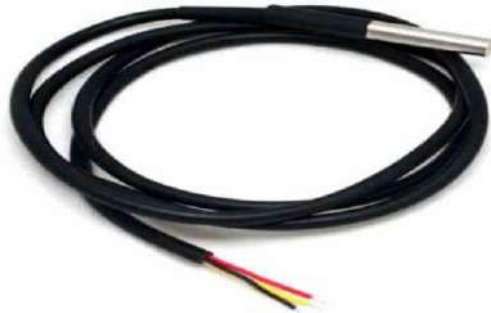
Figure 5.5 DS18B20 Temperature Sensor
