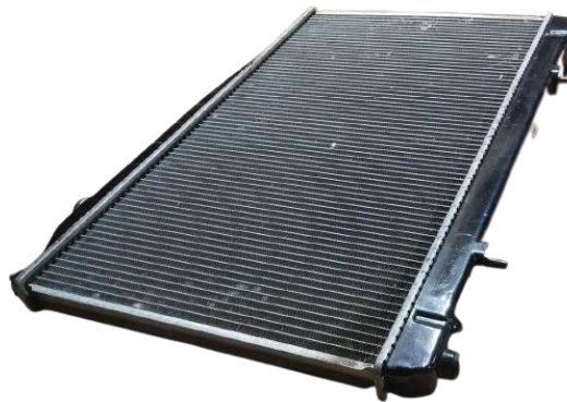
Figure 6.7 Heat Exchanger (Radiator)
