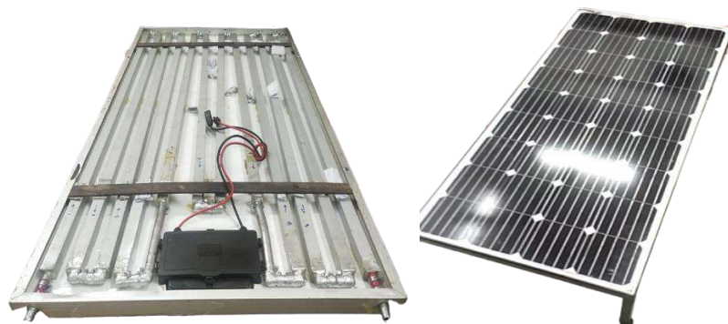
Figure 3.3 Heat Exchanger and Solar Panel
