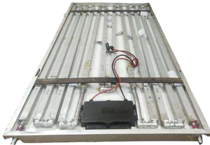
Figure 5.13 Heat Exchanger One (Rare Side of the PV Panel)
