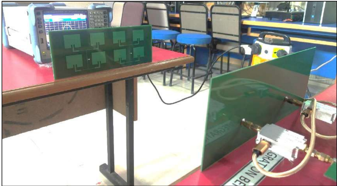
Figure 4-5: Integrated two 2x2 matrices form at both Tx and Rx ends
