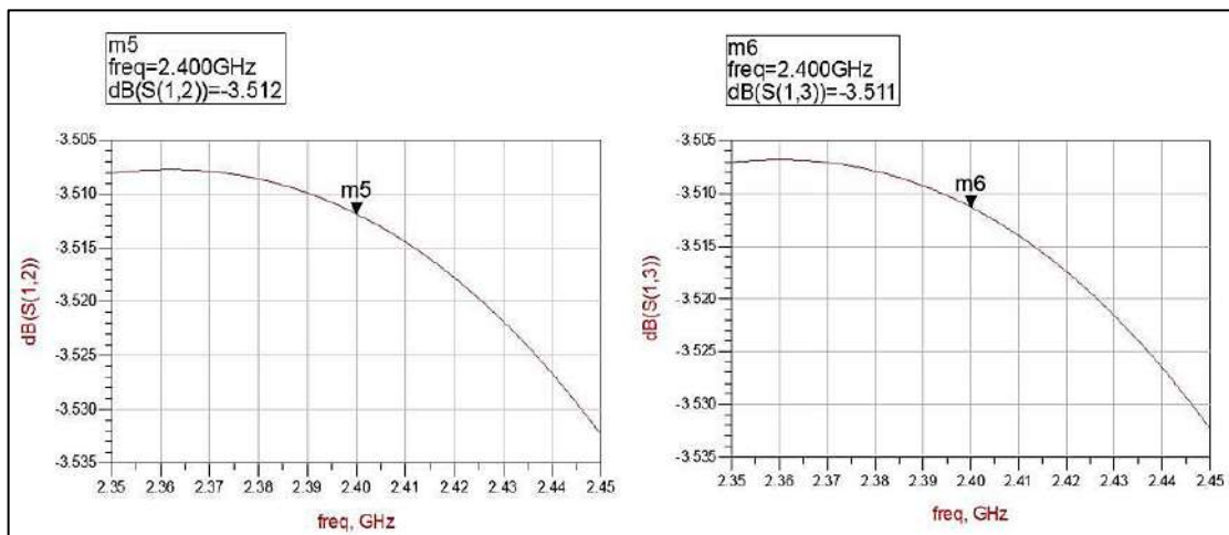
Figure 2-6: Simulated S12 and S13 parameters of 1x2 RF Power Divider
