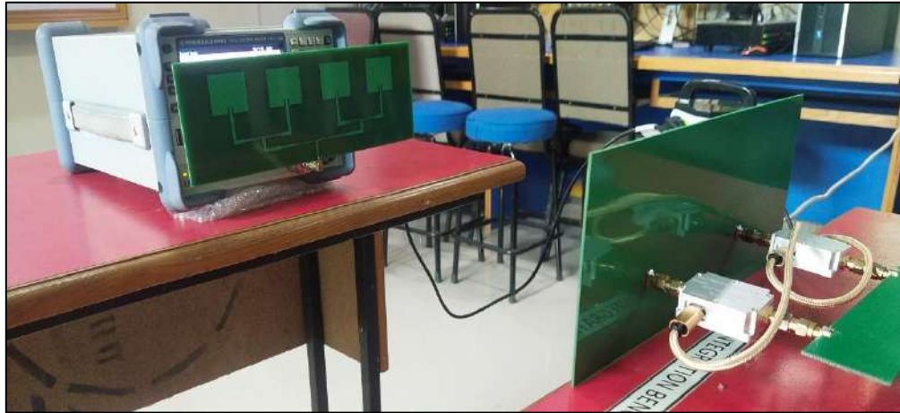
Figure 4-3: Integrated two 2x2 matrices form at Tx and Four Elements Array Form at Rx end
