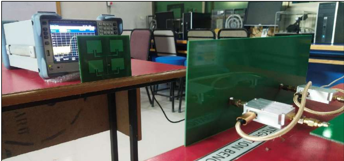
Figure 4-4: Integrated two 2x2 matrices form at Tx and 2x2 Matrix Form at Rx end
