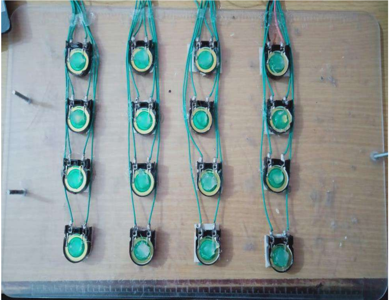
Figure 4.4 Arrangement of piezoelectric in the proto type tile
