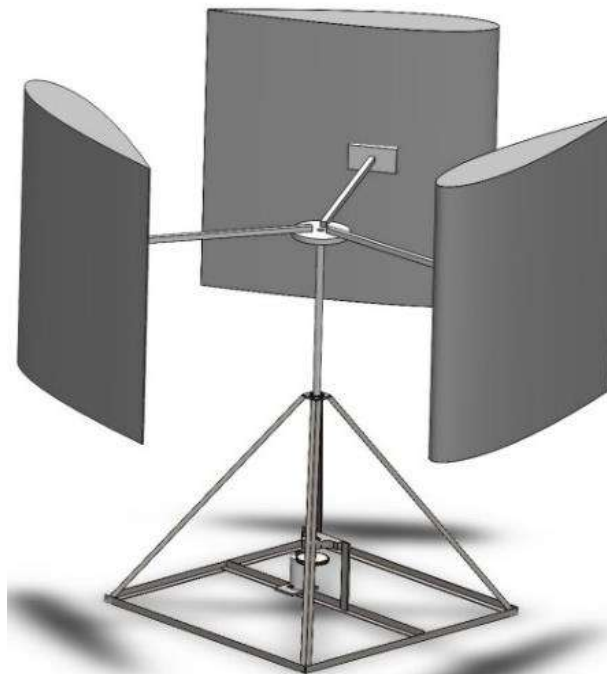
Figure 9 CAD Model of H-rotor VAWT using SolidWorks
