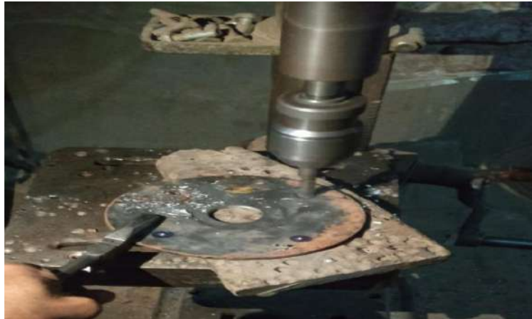
Figure 26 Drilling process on hub
