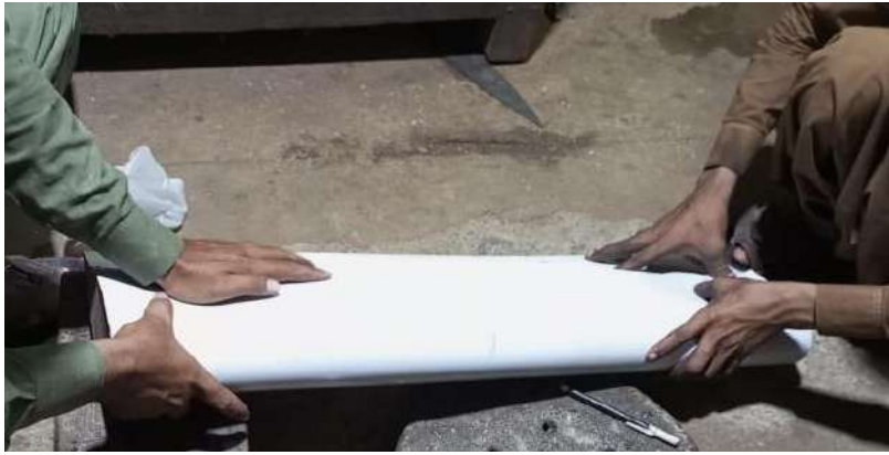
Figure 24 Bending of aerofoil sheet
