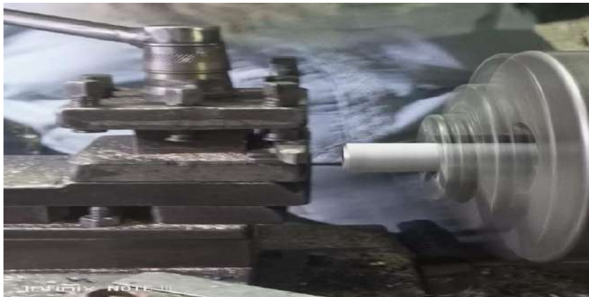
Figure 27 Facing process o shaft
