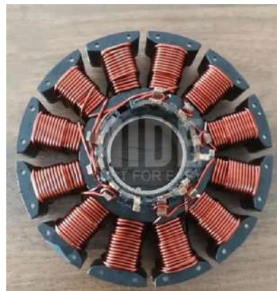
Figure 3.2 (b) Slotted Motor Windings Arrangement
