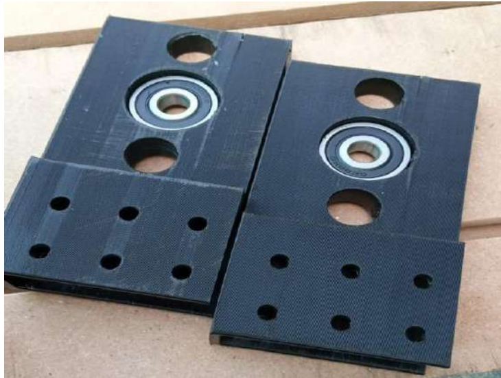
Figure 44: Bearings in 3d printed parts
