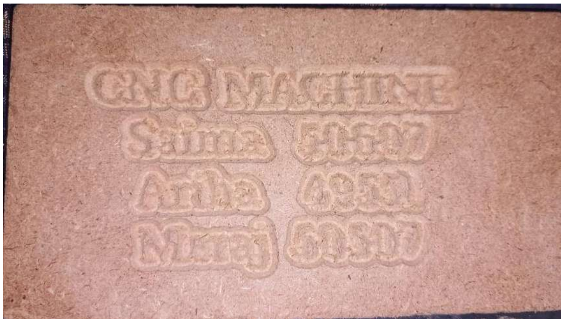
Figure 49: Engraved output on Wood
