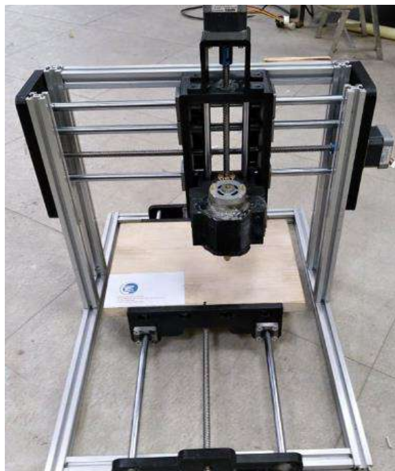
Figure 5: Final fabricated prototype milling machine assembly
