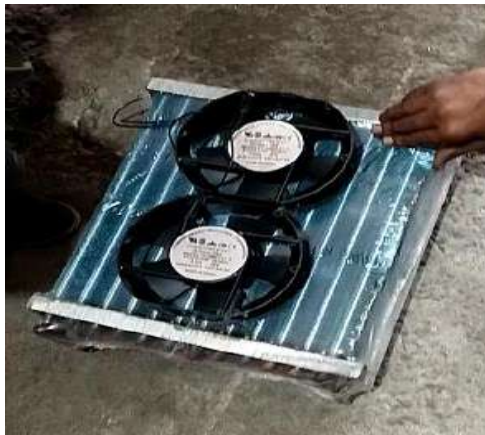
Figure 30: Fans on condenser
