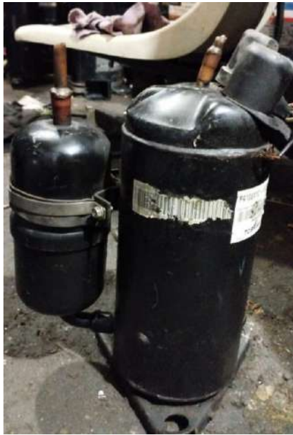
Figure 27: Scroll Compressor of r410a one ton capacity
