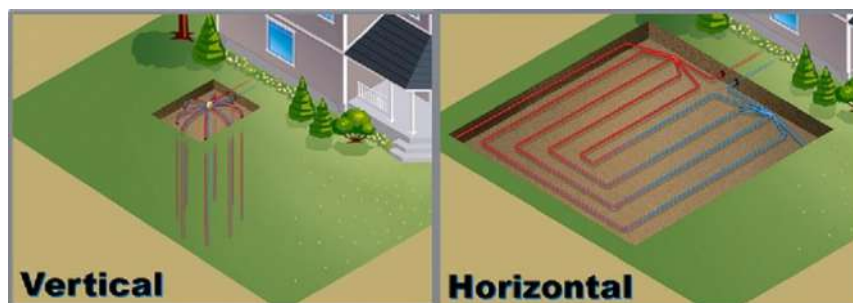
Figure 4: Ground-Source Heat Pumps
