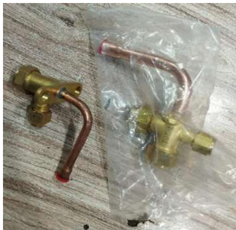
Figure 34: Service Valves for Spray of Refrigerant Inside the System
