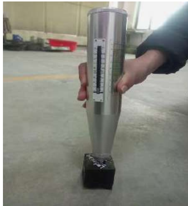
Fig. 16 Rebound Hammer Test
