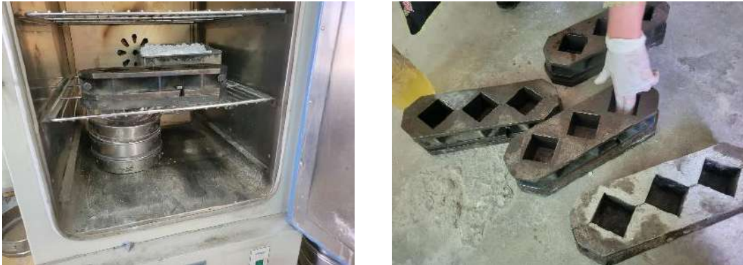
Fig. 7 Preheating of molds
