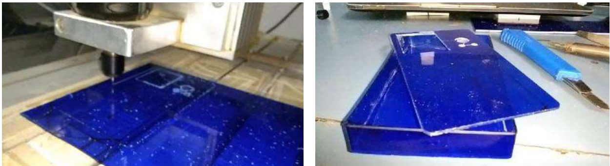
Figure 3.19: Design cutting of the casing of control unit.
