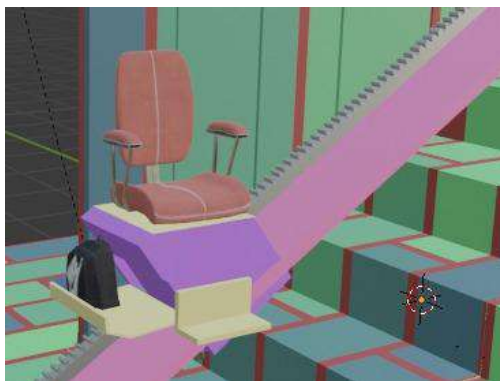
Figure 3.12 a: 3D design of stair lift
