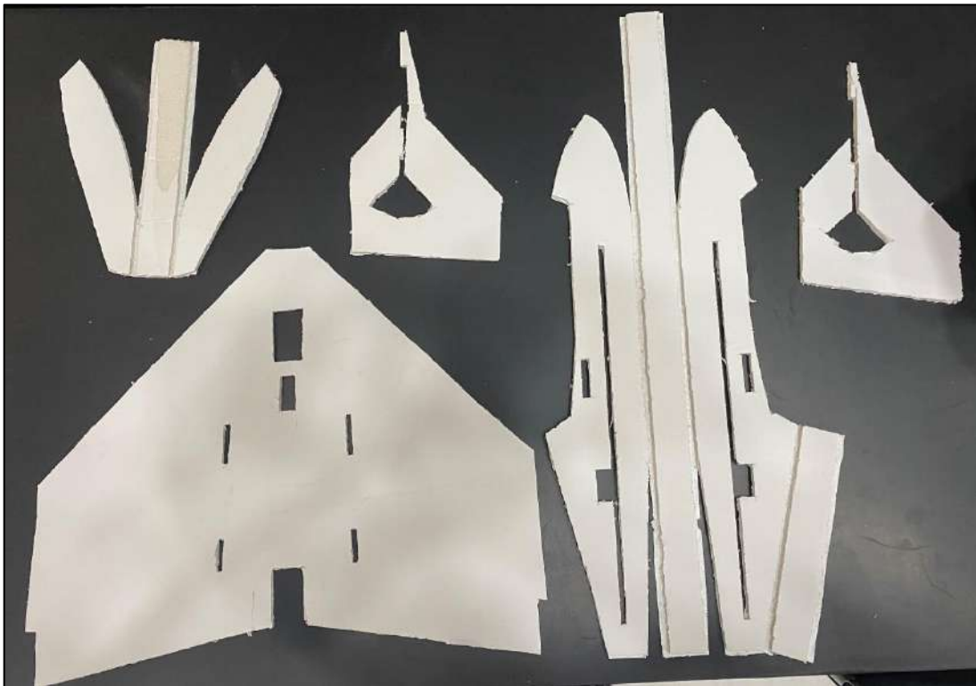
Figure 56:Fabricated parts for daughter plane
