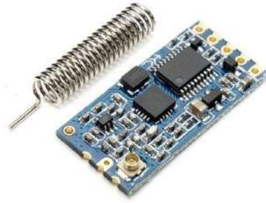
Figure-4.10 Hc-12 wireless module
