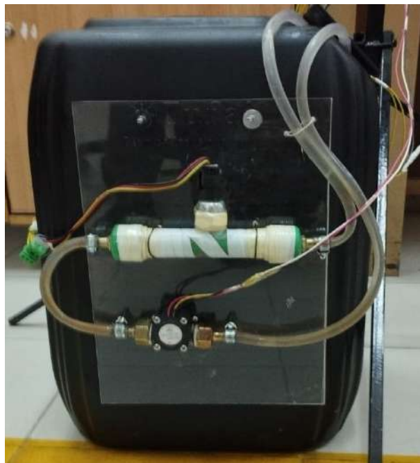
Figure 5.5 Tank with Sensors Mounted on it
