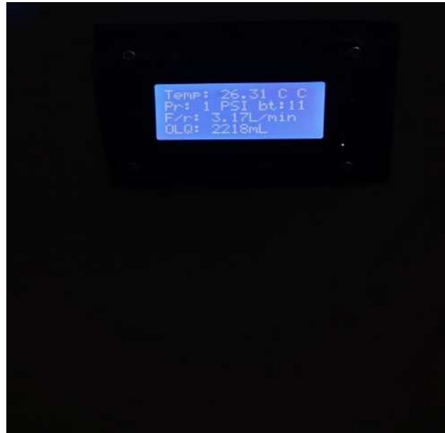
Figure 5.4 Parameters Values on the LCD Display on Monitoring Box
