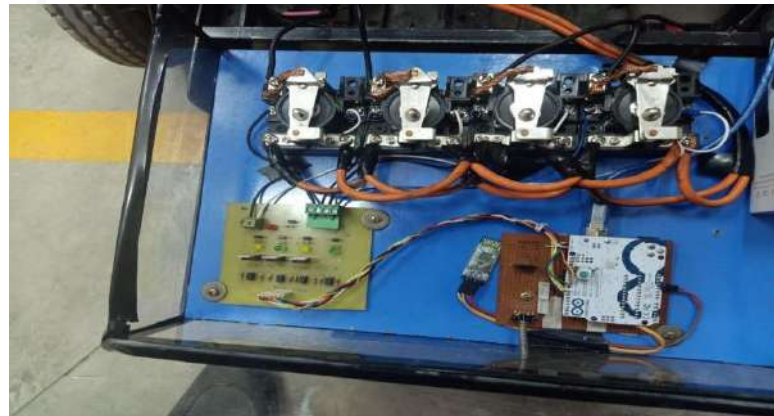
Fig 5.3 Relays Module implementation
