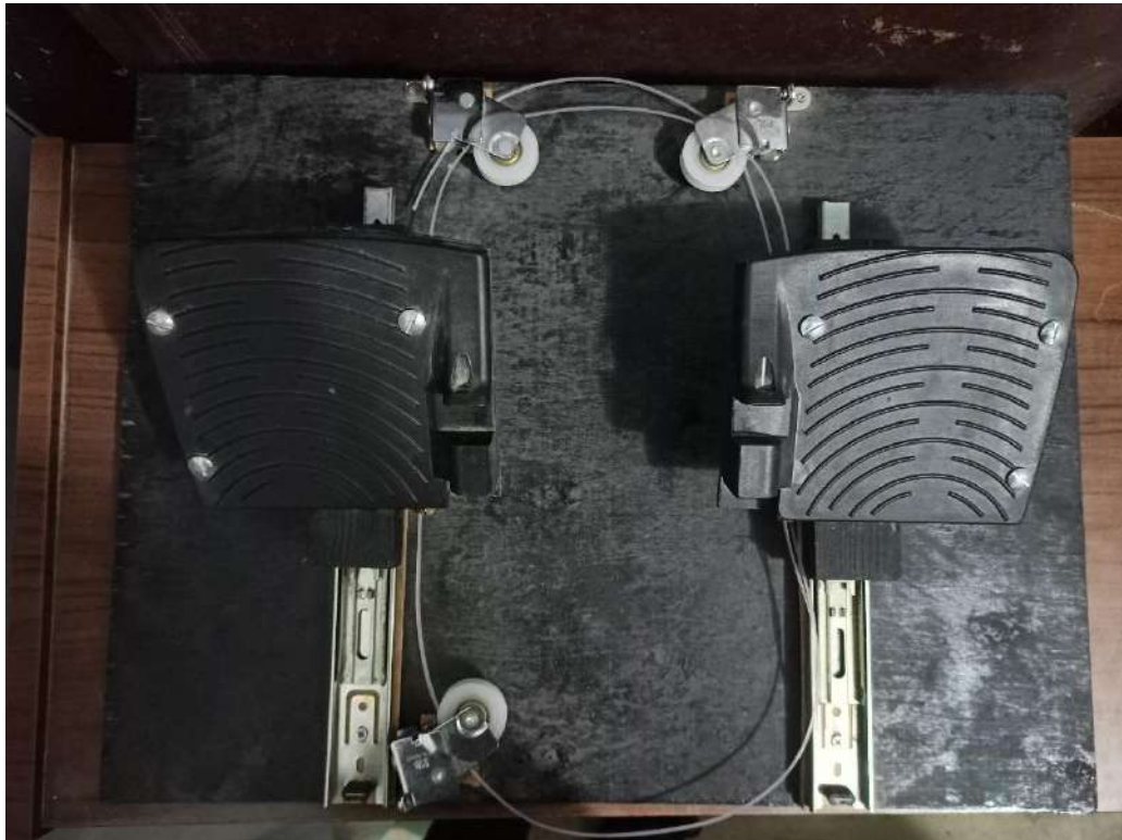
Fig 3-23: Final Assembly of Rudder Pedals
