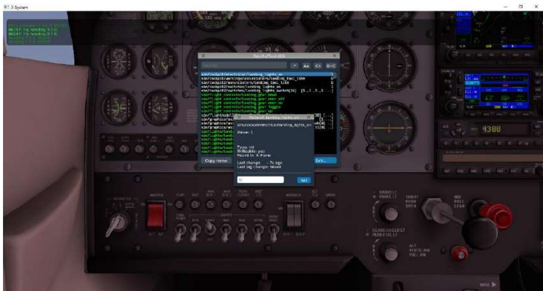
Fig 3-29: Controlling Landing Light Switch States using dataref
