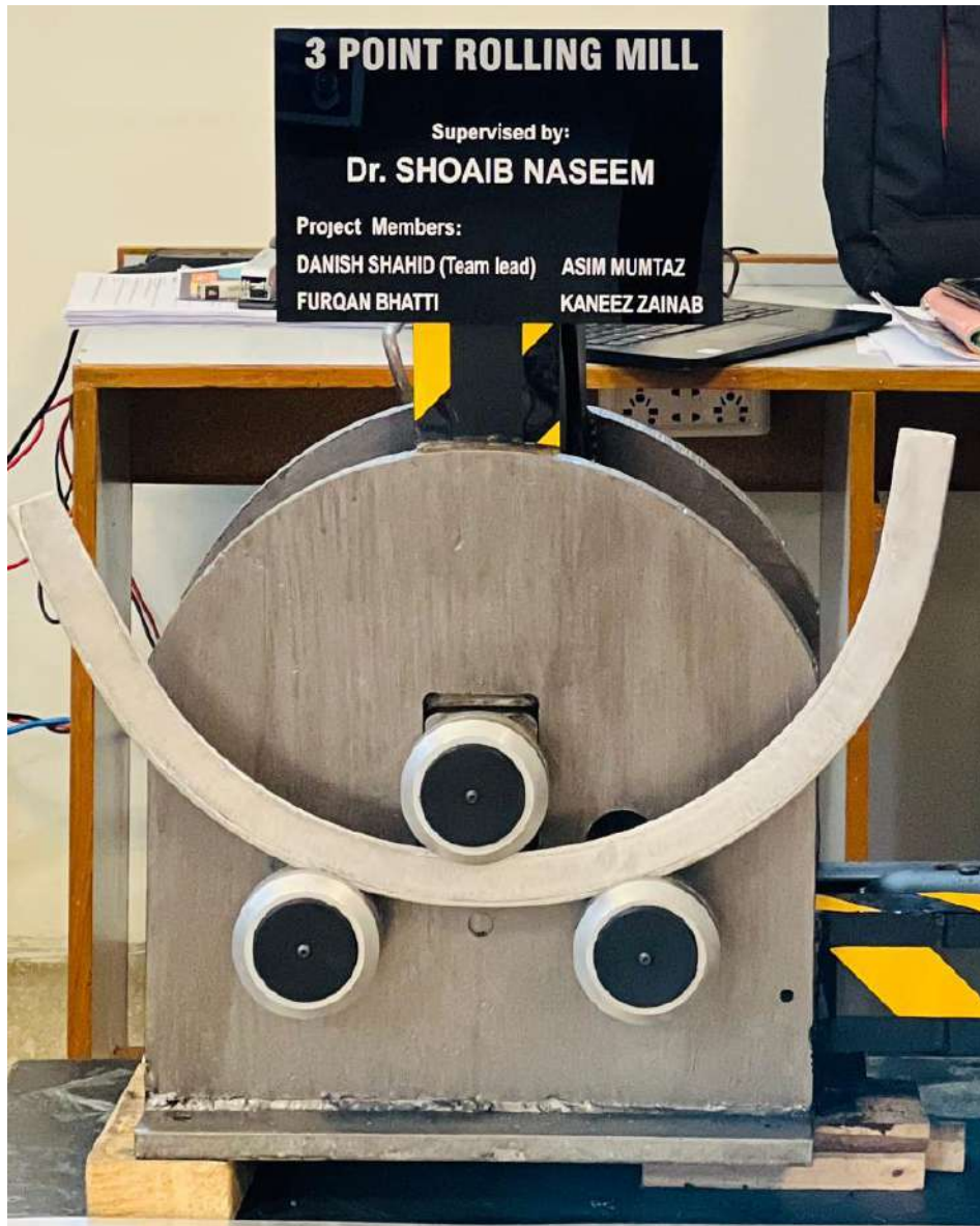
Figure 43 Rolling Mill After Assembly
