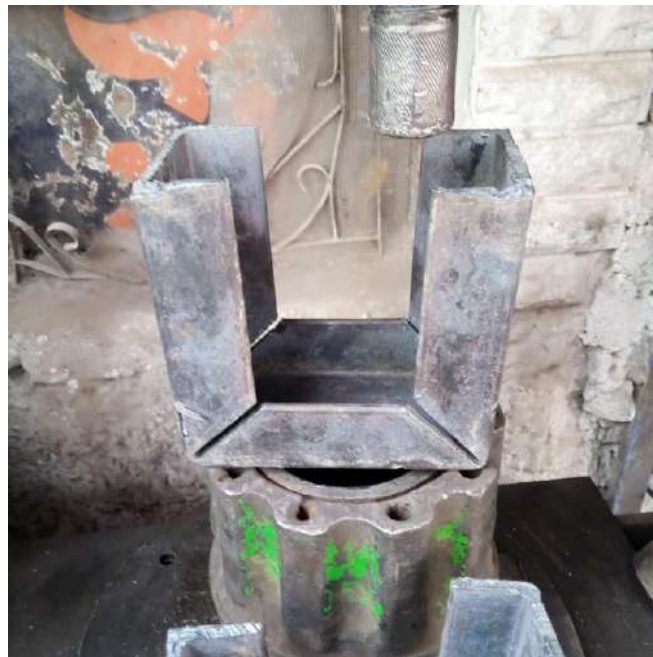
Figure 38 Hydraulic Housing during Its Fabrication
