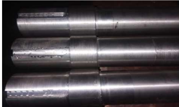
Figure 34 keyways Cut into the Shafts
