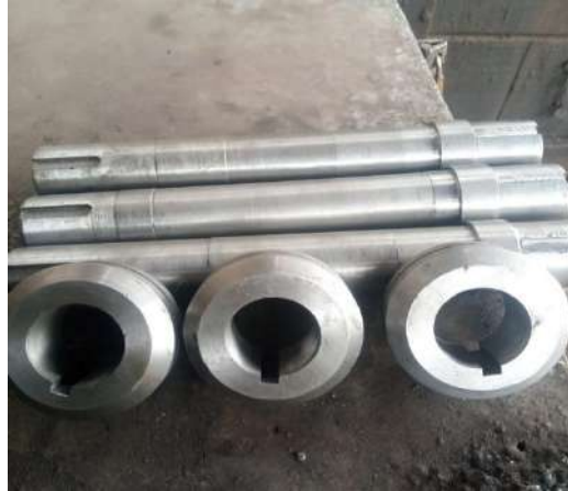
Figure 32 Shafts Behind the Rollers
