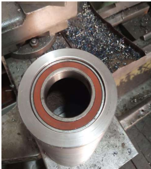
Figure 37 Shaft Housing with Bearing Installed
