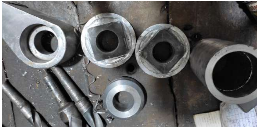
Figure 36 Sliders Along with Shaft Housing, Roller, and Swing Arm can be Seen
