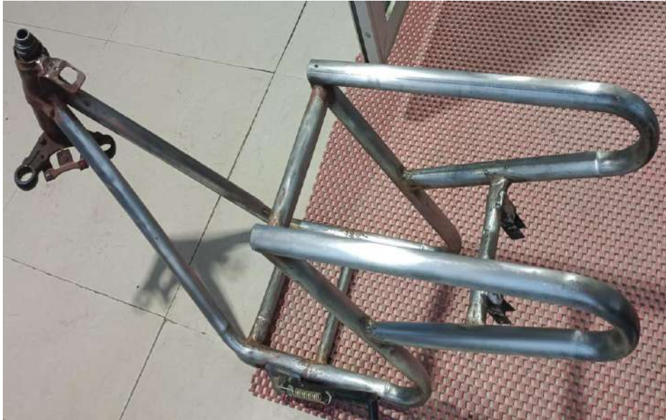
Fig 4. 8 Grinding Finishing for paint.
