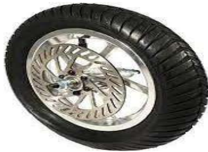
Fig 3. 25 Front Wheel of E-Bike with Disc
