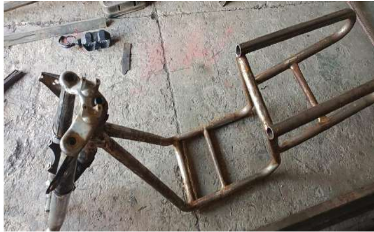
Fig 4. 2 With Pipes Final Assembled Frame
