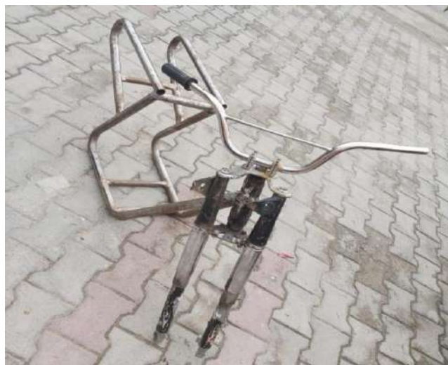
Fig 4. 3 Frame mounted with front handle and suspension
