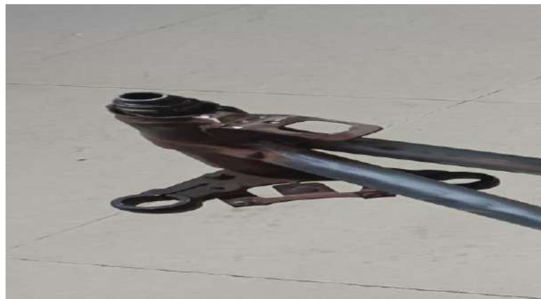
Fig 4. 5 Key Switch and Horn Mount
