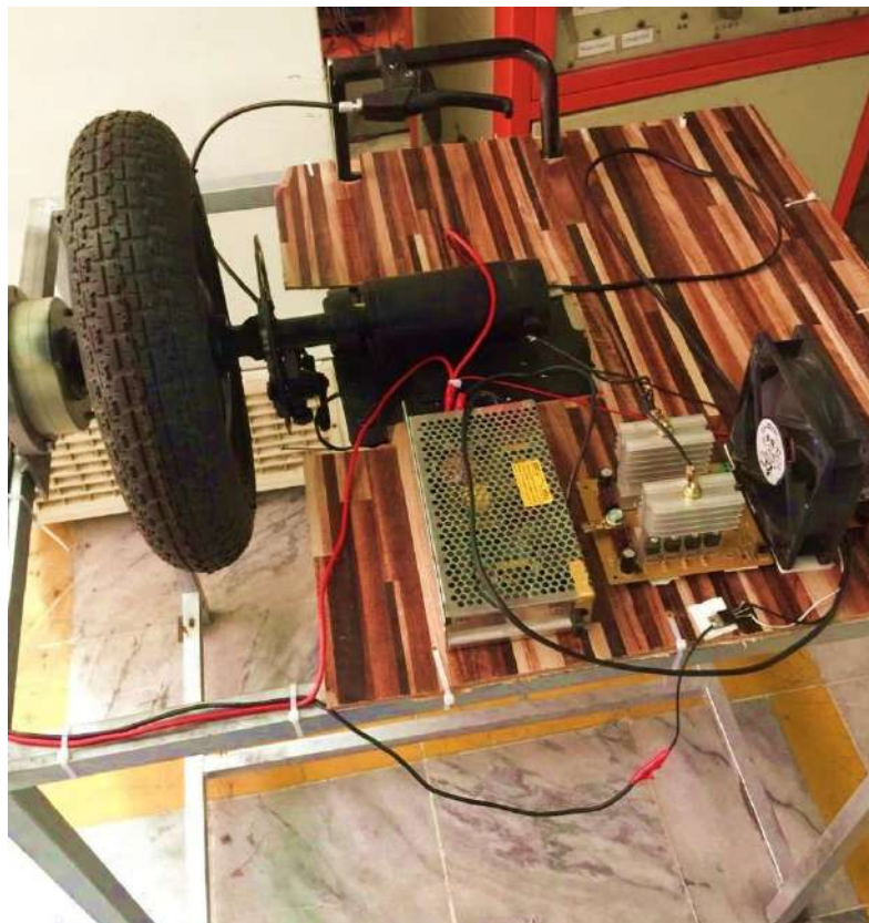
Figure 3-22: Experimental Model of Electromagnetic Braking System
