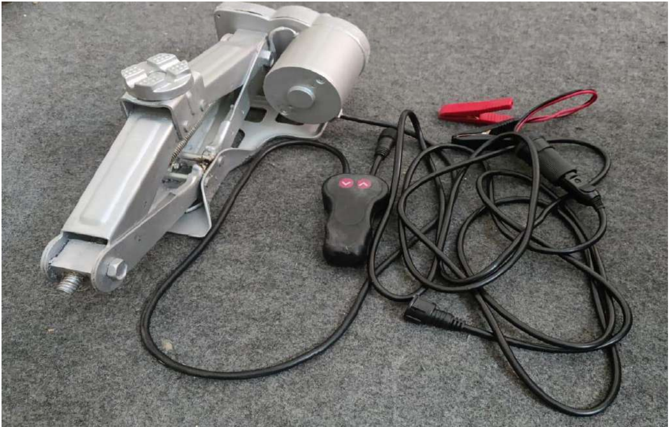
Figure 4 9: Fabricated Mechanized Automobile Jack
