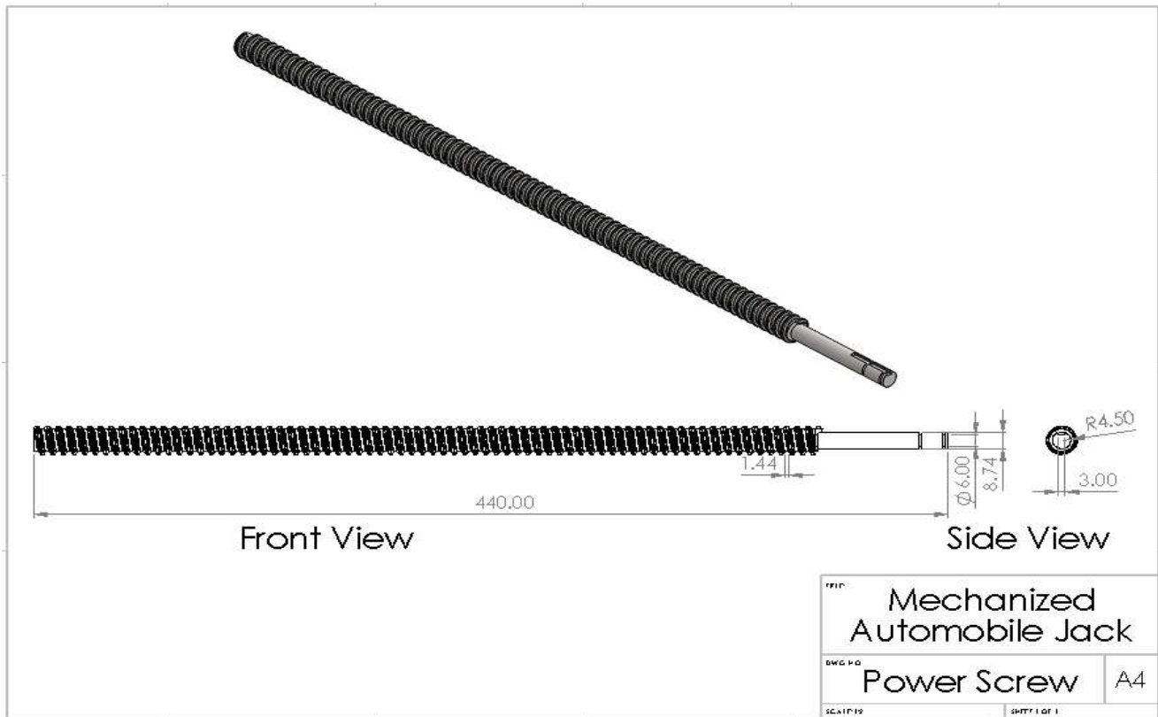
Figure 4 6: 2D detail Drawing of Power Screw
