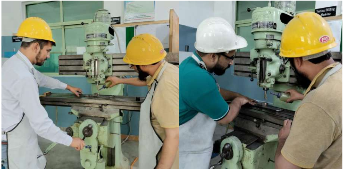
Figure 3.11: Manufacturing Parts on Milling Machine
