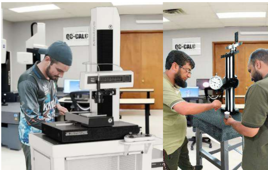
Figure 4.1: Experimental Verification Procedures on Digital Surface Tester and Dial Indicator on Granite Surface Table
