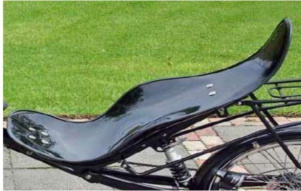
Figure 3-27: Recumbent trike seat
