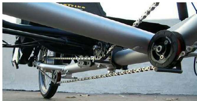
Figure 3-20: Chain drive with idlers
