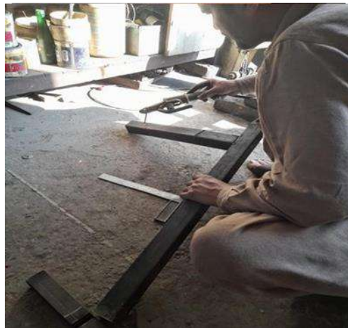
Figure 3-30: Welding of chassis.
