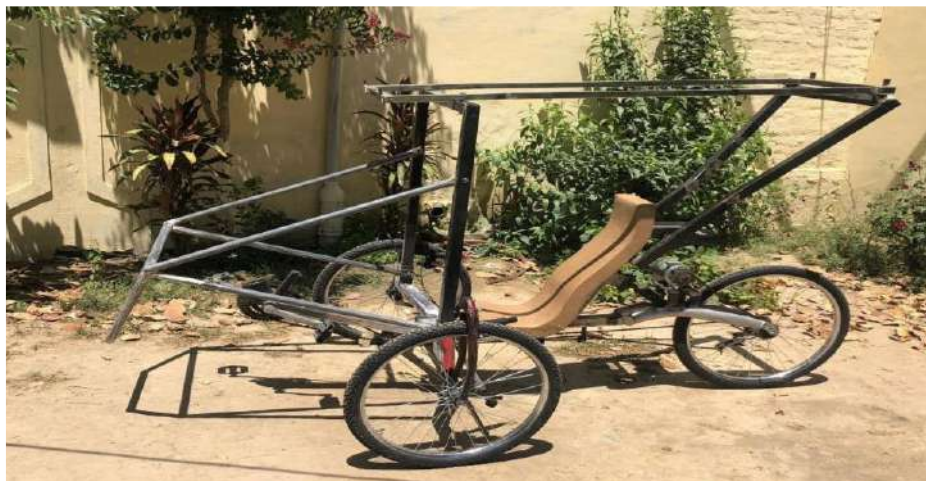
Figure 3-38: Fabricated Model of Project
