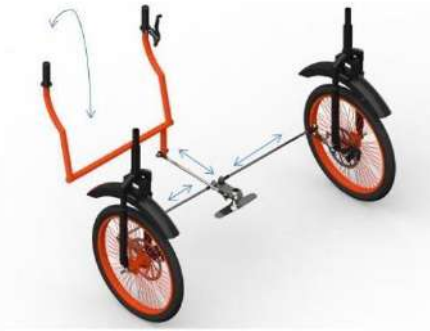
Figure 3-24: Simple push and pull type steering
