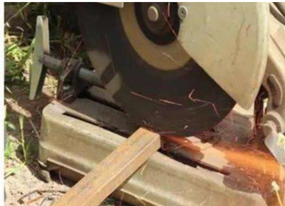
Figure 3-28: Disk Cutting of cast iron for trike
