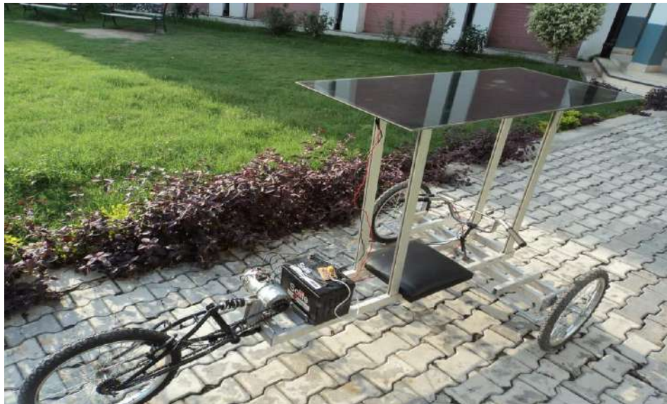
Figure 1-2: Solar power recumbent trike
