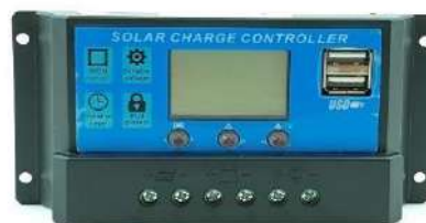
Figure 3-26: Solar charge controller
