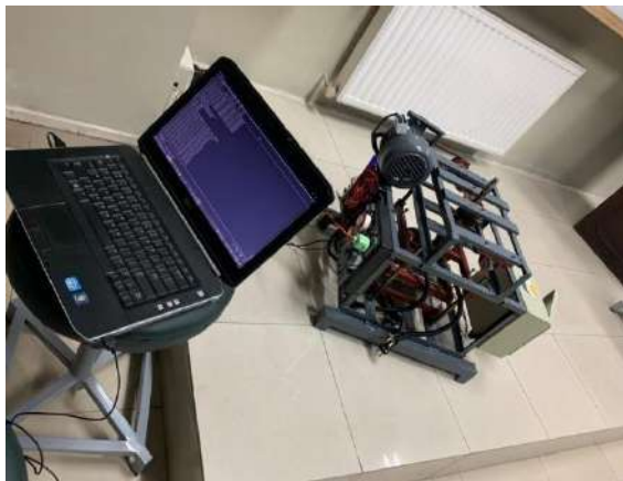
Figure 4.23: Heat press operating and data recording via Arduino serial monitor
