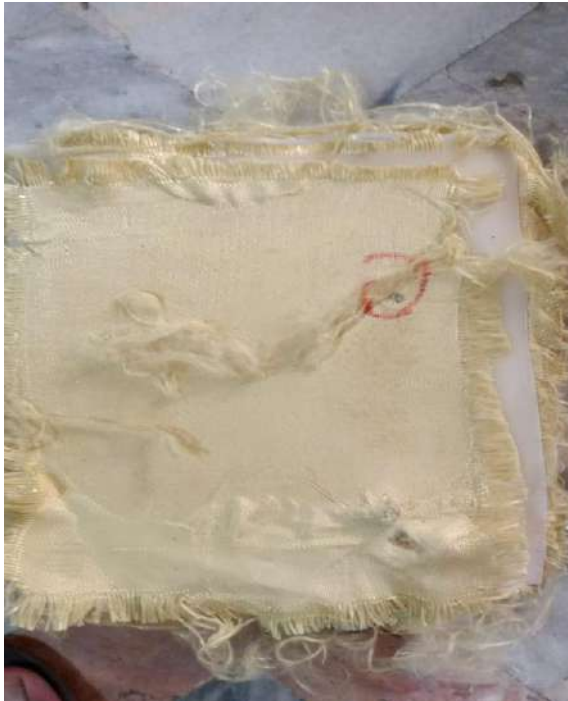
Figure 5.5: Combined samples tested with a single fire. (Distance 15 ft / 9 mm round)
