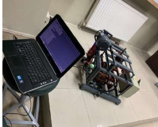
Figure 5.2: Heat press operating and data recording via Arduino serial monitor
