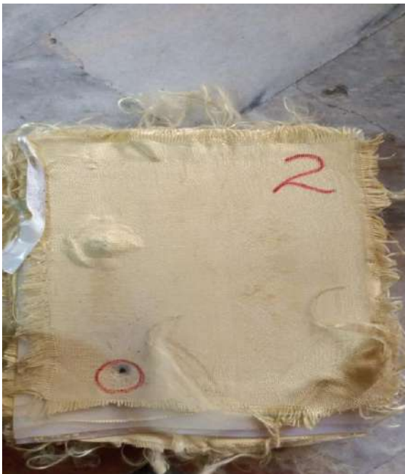
Figure 5.7: Second sample tested with a single fire. (Distance 15 ft / 9 mm round)
