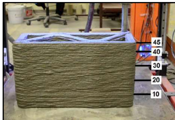
Figure 2.3: 3D Printed Structure of The Wall.
