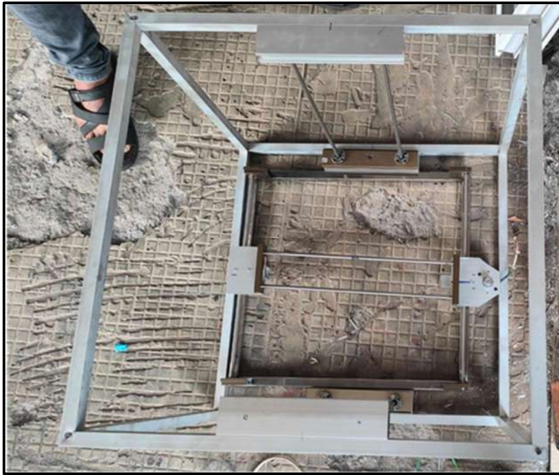
Figure 4.5: Gantry System without Motor Installation
