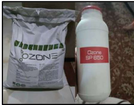
Figure4.21: Silica Fume and Accelerator for Concrete Mixture
