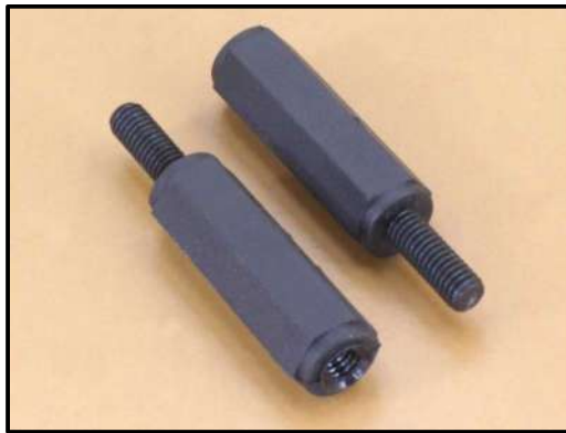
Figure 4.10: Screw PCB Standoffs Hexagonal Spacers M3 Male x Female 40mm
