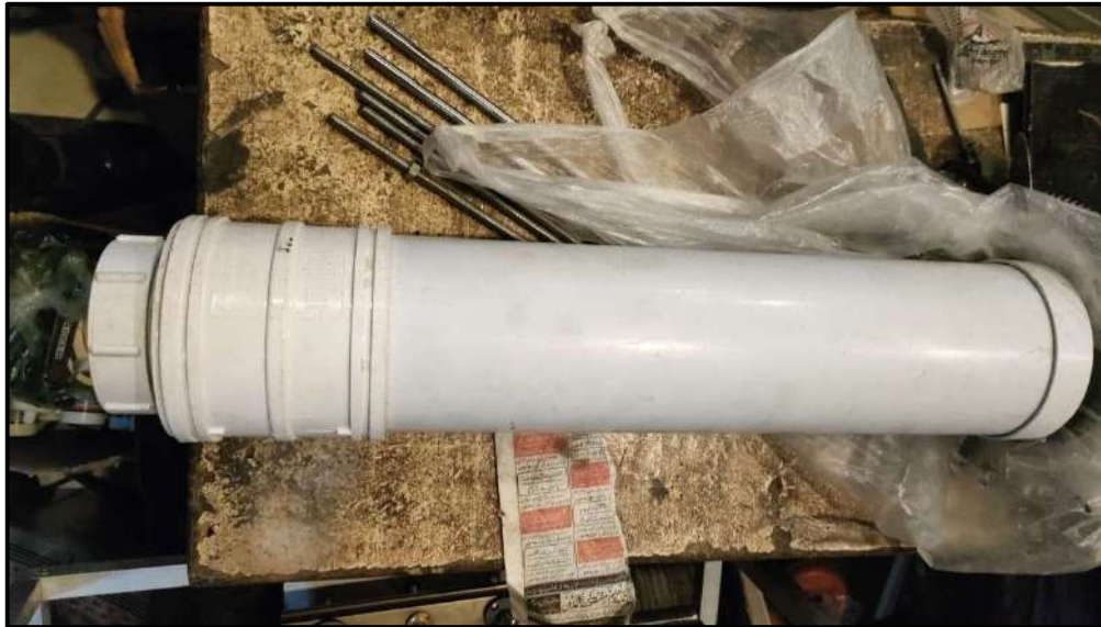
Figure 4.8: PVC Pipe Extruder with Rubber Inside for Concrete Extrusion
