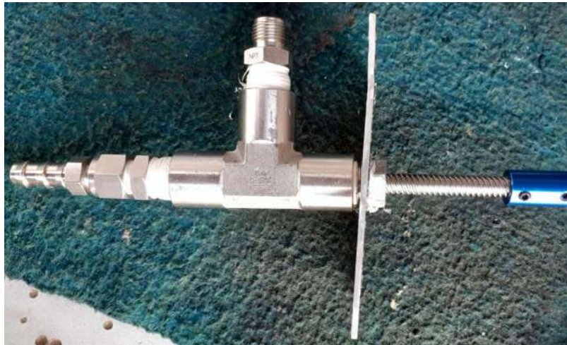
Figure 4.12: The Final Fabrication of The Nozzle with Motor Mounting Plate and Coupling
