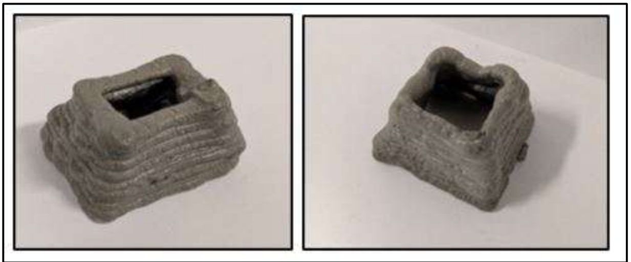
Figure 4.24: (a) The 3D Printer Pyramid-Like Shape (40 × 20mm) (b) The 3D Printer Pyramid-Like Shape (40 × 40mm)
