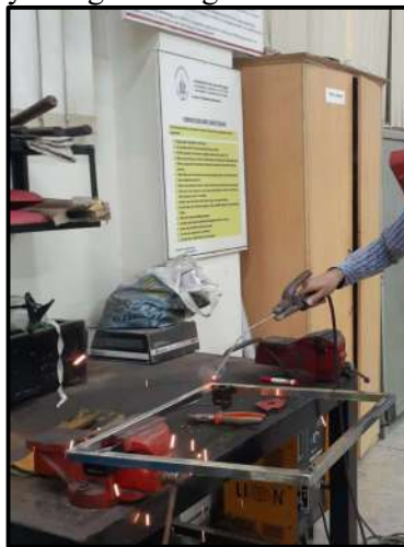
Figure 4.2: Welding for Stainless Steel Frame and Motor Brackets
