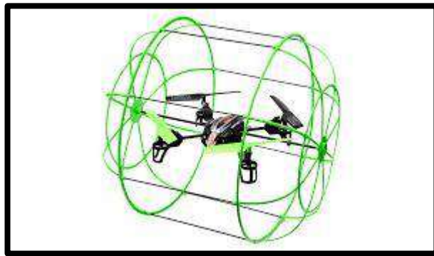
Figure 2.9 Add-on Drone Cage
