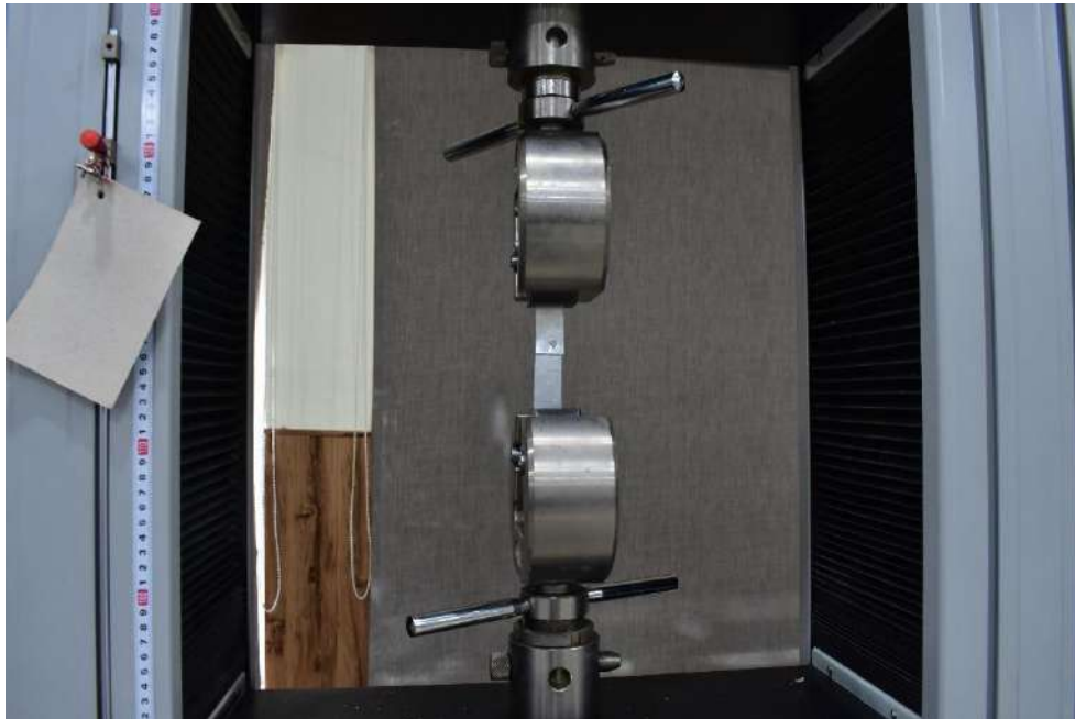
Figure 12: sample in ultimate tensile testing machine
