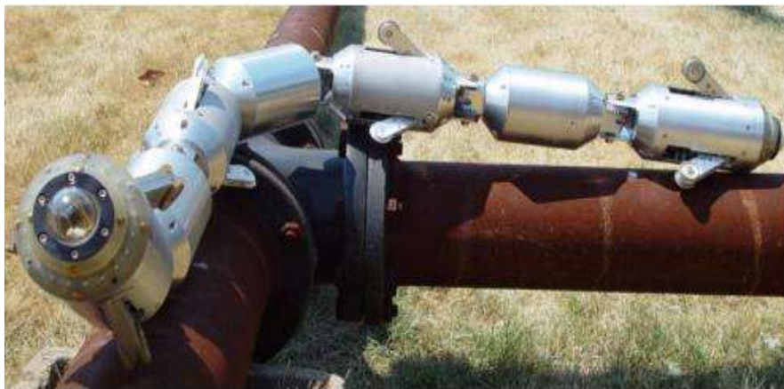
Figure 1-9: Prototype of the X-I Explorer robot originally designed at Carnegie Mellon University. Image from [25].
