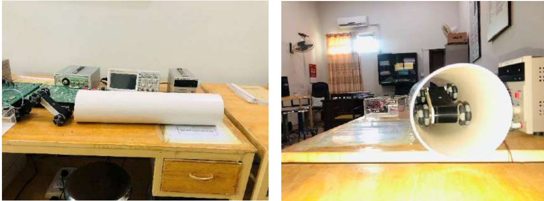
Figure 4.3 Driving robot forward and backward in horizontal straight pipe
