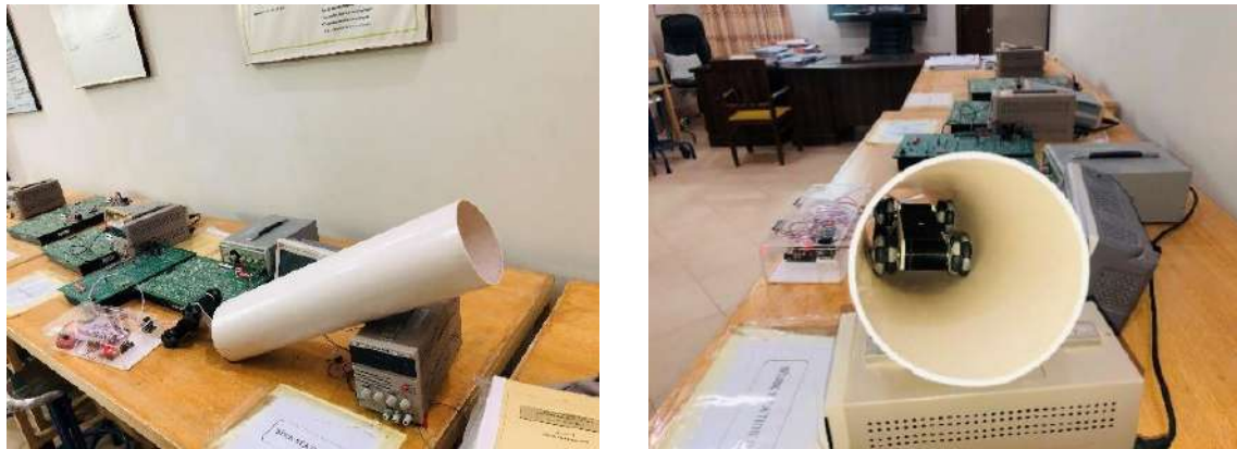
Figure 4.5 Driving up and down in straight pipe inclined at 60 degrees from the earth surface.
