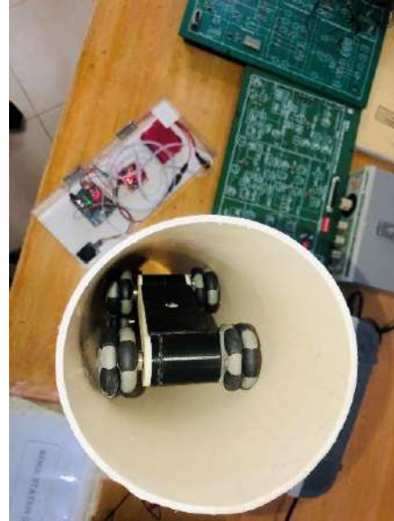
Figure 4.6 Driving up and down in vertical straight pipe inclined at 90 degrees from the earth surface
