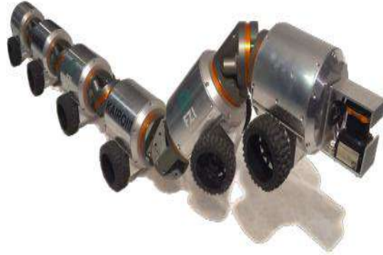
Fig. 1.11. The modular snake-like inspection robot KIRO 3 (image from [34])
