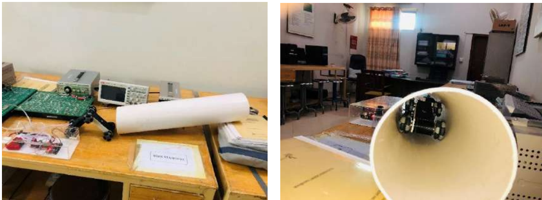
Figure 4.4 Driving up and down in straight pipe inclined at 30 degrees from the earth surface.
