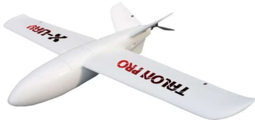
Figure 5: Fixed wing UAV with V tail [11]
