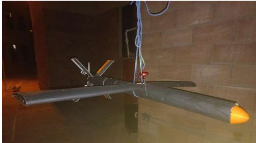
Figure 79 Center of Gravity Testing
