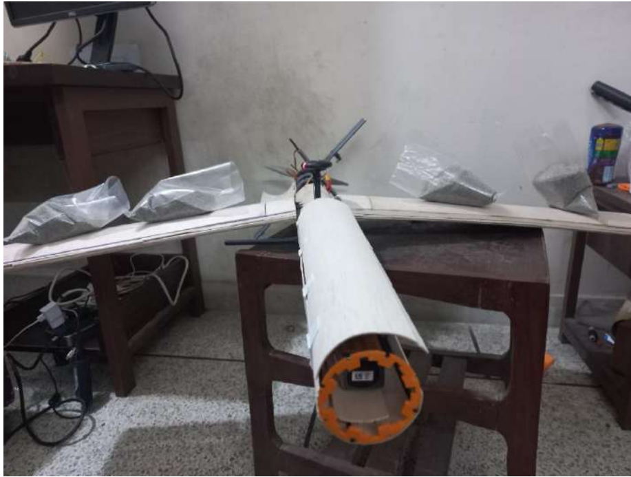
Figure 77 Static Wing Loading Test
