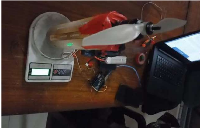
Figure 78 Motor Thrust Testing
