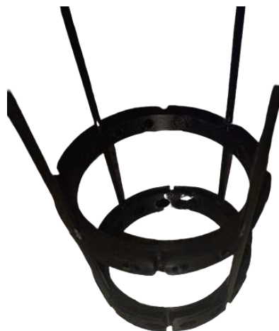
Figure 74 Carbon Fiber Stringers attached to Formers
