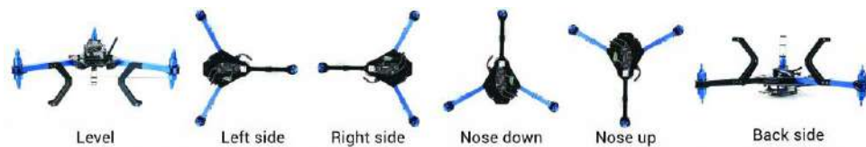
Figure 64: Accelerometer Calibration positions
