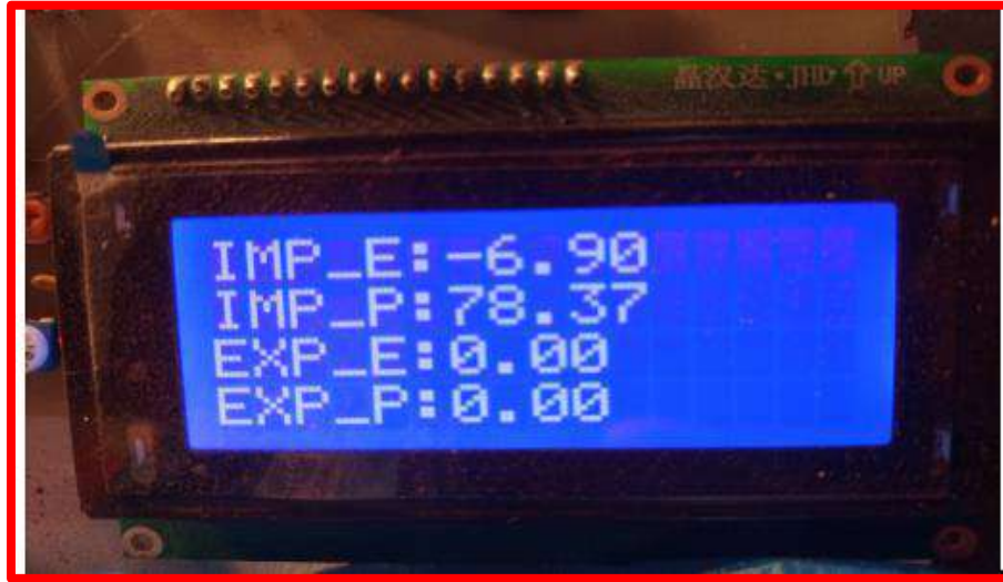
Fig 6.3 Output When 480 W Load is Connected
