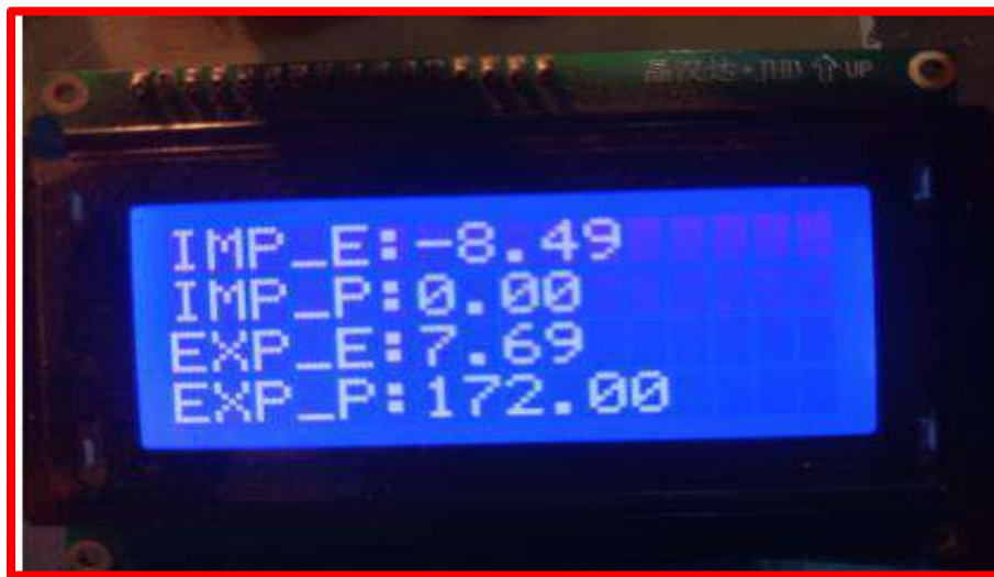
Fig 6.6 Output When 200 W Load is Connected
