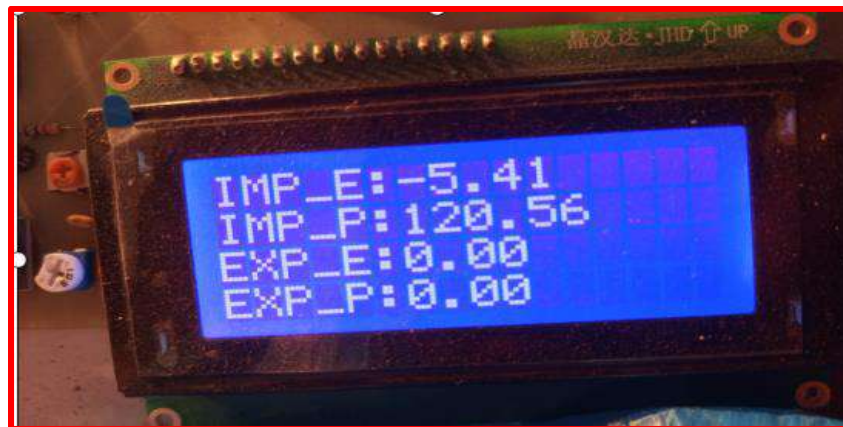
Fig 6.2 Output When 520 W Load is Connected
