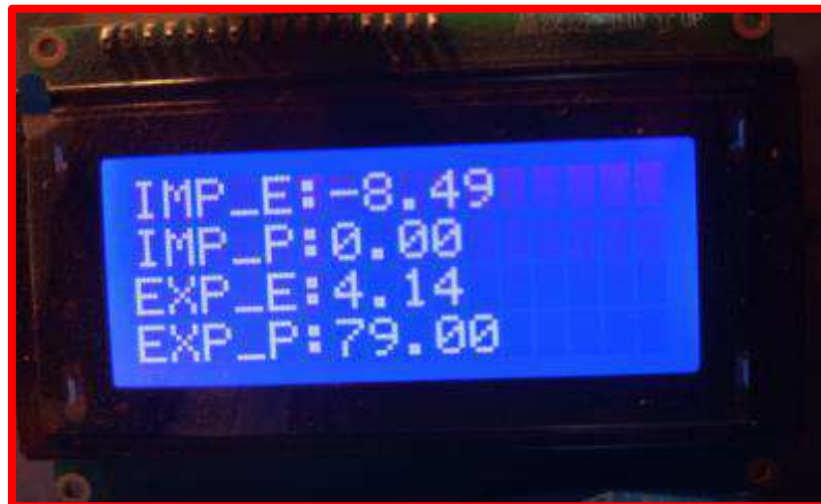
Fig 6.4 Output When 300 W Load is Connected
