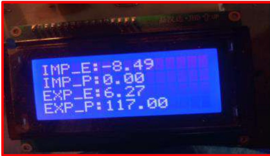
Fig 6.5 Output When 260 W Load is Connected
