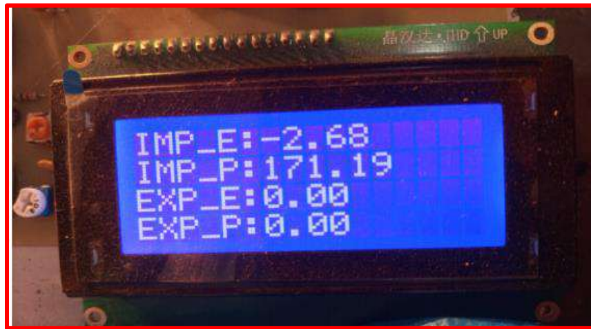
Fig 6.1 Output When 580 W Load is Connected
