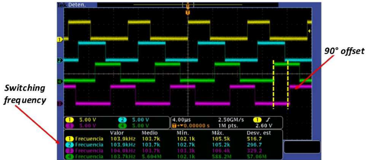
Figure 4. Commutation signals for phases with the corresponding 90° phase shift and duty cycle (40%40%)
