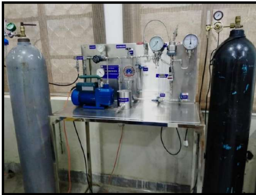
Figure 3-6 Gas Permeation Setup in Department of Polymer and Process Engineering (Polymer Synthesis Lab), UET Lhr
