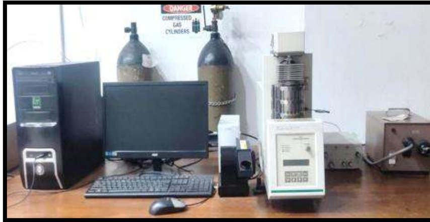
Figure 3-8 Thermogravimetric analysis Setup in Department of Polymer and Process Engineering (Polymer characterization Lab), UET Lhr
