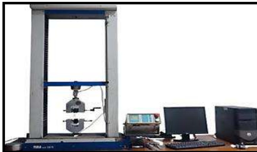
Figure 3-9 Universal testing machine Setup in Department of Polymer and Process Engineering (Polymer characterization Lab), UET Lhr
