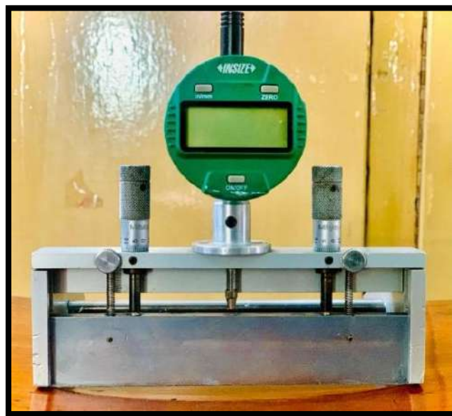
Figure 3-3 Doctor blade in Department of Polymer and Process Engineering (Polymer Composite Lab), UET Lhr
