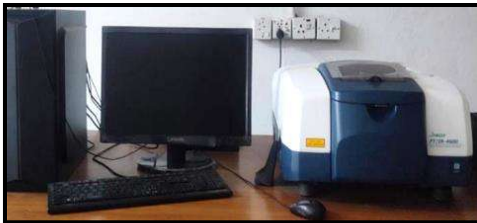
Figure 3-7 Fourier Transmission infrared spectroscopy (FTIR) in Department of Polymer and Process Engineering (Polymer Characterization Lab), UET Lhr
