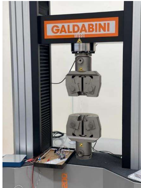
Figure 17: Electrical circuit and mounted near the UTM machine
