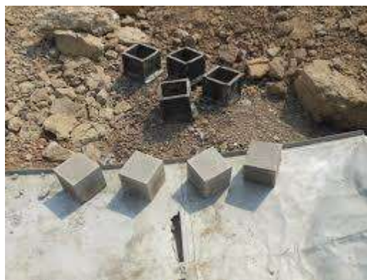
Fig.3.13. Demolding of Cubes.
