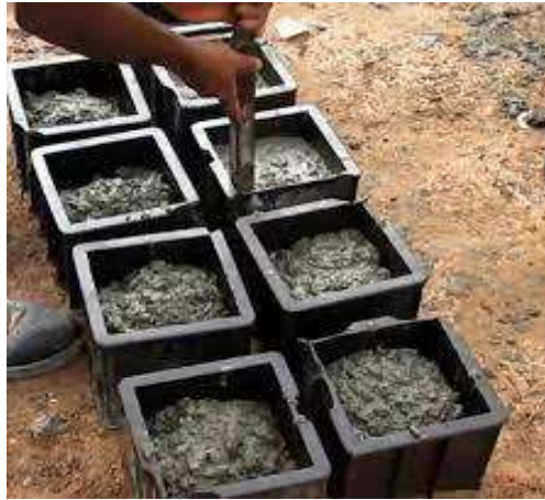
Fig.3.12. Pouring concrete paste into cubes.
