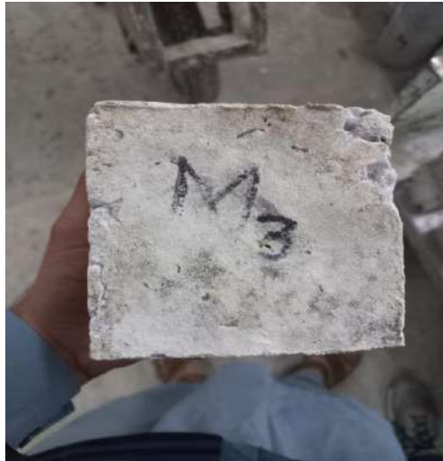
Fig.3.14. Demolded cubes for testing.
