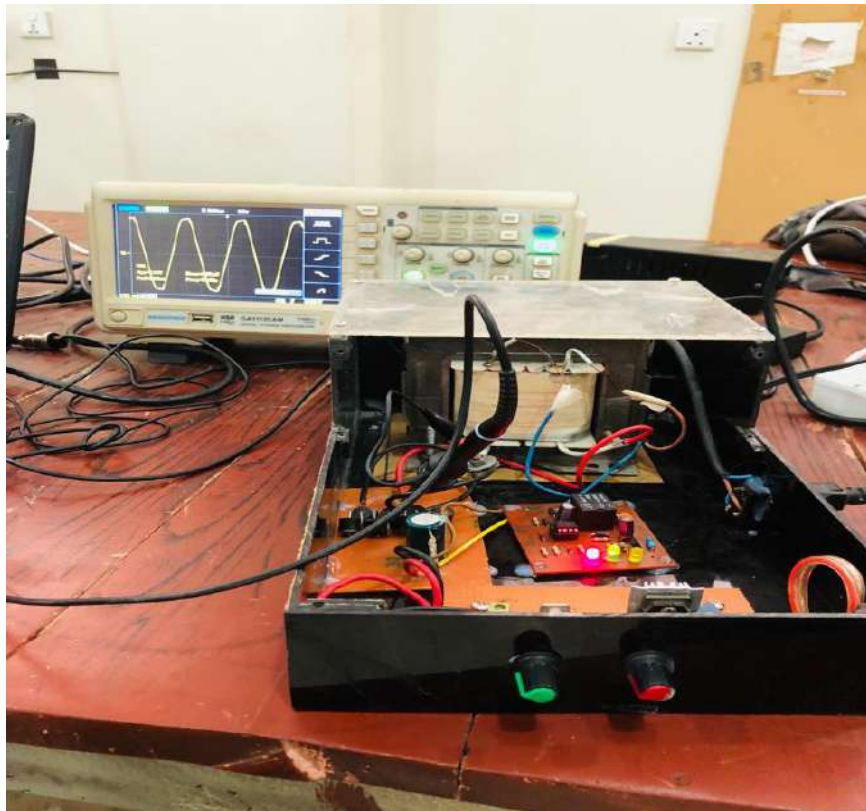
Figure 5.2 Sinewave of transformer
