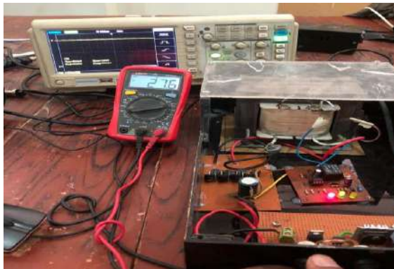
Figure 5.4 Output of the Bridge Circuit
